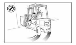
Do not start, stop, turn or change direction suddenly or at high speed. Sudden movement can cause the lift truck to tip over. Slow the speed of your truck and use the hom near corners, exits, entrances, and near people.
