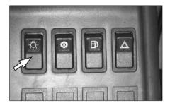
This switch changes over the modes of the inching control pedal, inching and no-inching.
