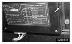
ASC-200/201 has internal indicator on the right side of the controller for displaying the selected gear and the abnormal condition.
