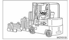
Use special care when operating on grades. Do not angle across or turn on grades. Do not use a lift truck on slippery grades. Travel with forks downgrade when unloaded. Travel with load upgrade.
