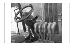
The mast can be tilted by operation of this tilt lever. Pulling on this lever backwards will tilt the mast backwards, and pushing it forwards will tilt the mast forwards. The tilt speed can be controlled by tilt angle of the lever and accelerator pedal effort.
