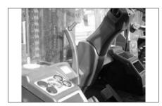
The parking brake lever is located at the left side of the steering wheel.
