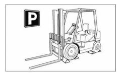
Park your lift truck in authorized areas only. Fully lower the forks to the floor, put direction lever in NEUTRAL position, engage the parking brake, and turn the key to the OFF position. Remove the key and put blocks behind the wheels to prevent the truck from rolling. Shut off your forklift truck when leaving it unattended.
