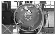
NOTE: If a LP equipped lift truck is stopped or parked for an indefinite or prolonged period of time, close the fuel shutoff valve on the LP tank. Run the engine until fuel in the line runs out and the engine stops. Turn off the ignition switch and disconnect switch (if equipped).
