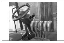
The forks can be raised or lowered by pulling backwards or pushing forwards on this lever. The lift speed is controlled by tilt angle of the lever and accelerator pedal effort. The lowering speed can be controlled by tilt angle of the lever. The engine speed or accelerator pedal has nothing to do with the lowering speed of the forks.
