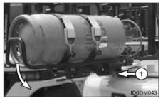
Pull the release knob (1) and then push down the tank.
