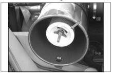
Remove the secondary element. Inspect the gasket between the air cleaner housing and the engine inlet. Replace the gasket if it is damaged.
