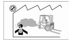
Exhaust from all internal combustion engines contains carbon monoxide, a colorless, odorless, tasteless, poisonous gas. Exposure to carbon monoxide can cause serious injury or health problems, including death. and avoid unnecessary idling of the engine. If nausea, dizziness or headaches are experienced stop the truck and seek fresh air.
