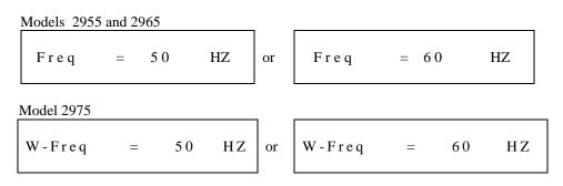
Press the Up or Down Arrow keys to toggle the frequency selection; 50 or 60 hertz, then press the EXIT key to exit to the test mode or toggle to another setting using the SET key.
