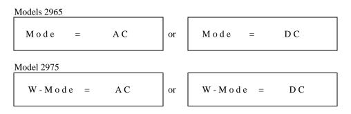
Press the Up or Down Arrow keys to toggle the output function; AC or DC, then press the EXIT key to exit to the test mode or toggle to another setting using the SET key.
