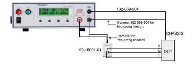
The adapter box allows you an easy way to connect an item which is terminated in a two or three prong line cord. If you are testing a product which is terminated in a three-prong plug, you are also required to perform a continuity or ground bond test on the ground conductor of the DUT to the chassis or dead metal of the product. With the 2900 models, you can perform both the hipot and continuity tests at the same time by activating the continuity function on the instrument.
