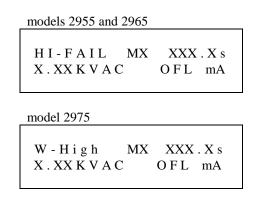
7. If the leakage current exceeds the metering range and neither a short circuit nor flash over occurred, the red indicator light will illuminate on the RESET switch and an alarm will sound. The display will show:
