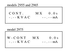
If you are not performing a Ground Continuity Check, the Ground Continuity must be set to the "OFF" (Disabled) position. It is not necessary to connect the "Cont.Check" cable since this test will not be performed if the circuit is disabled. The instrument will proceed with the Hipot Test when the "Test" switch is activated.
