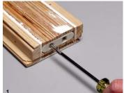
Pry the shoot bolt guide from the panel with a flat headed screwdriver or pry bar. See illustration 2.
