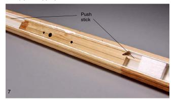
Thread the head jamb shoot bolt through the foam block as described in step 9 from previous section. See illustration 8.
