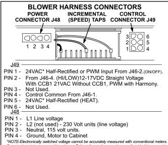
\*NOTE-Electronically switched voltage cannot be accurately measured with conventional meters. Do not attempt to measure this voltage. Follow diagnostic procedures outlined in this manual to determine if motor and VSP1 are operating properly.
