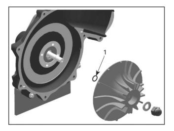
Inspect back of impeller if o-ring<sup>1</sup> is not on impeller shaft.
