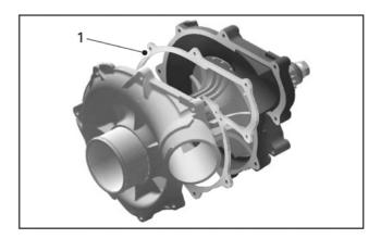
Spread evenly covering surface completely. Clean any excess sealant at inner edge of spacer so as to prevent sealant from discharging into impeller area when halves are joined together.
