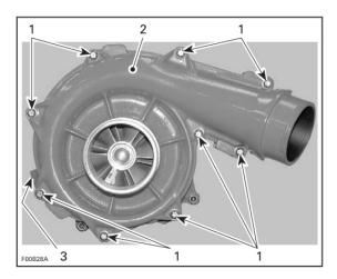
Remove impeller cover and discard. **NOTE:** It may be necessary to tap the cover in order to remove it. Use only a dead blow mallet and tap only on tab at top of impeller cover plate. **DO NOT PRY COVER OFF.**
