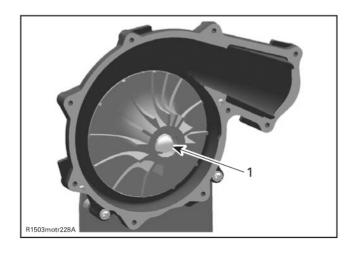
Carefully remove OEM impeller<sup>2</sup> by twisting and pulling. **NOTE:** Make sure o-ring<sup>3</sup> is in place against step collar on impeller shaft.
