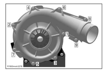
Spin impeller shaft to ensure smooth operation.
