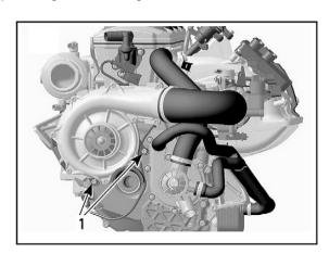
Remove the one M6 x 35mm Torx bolt<sup>1</sup> that secures rear of supercharger unit to engine. **NOTE:** You will need a special Torx adapter to remove and replace the upper/rear Torx bolt. This can be purchased through our parts department, a Sea•Doo Dealer, or a reputable tool company.
