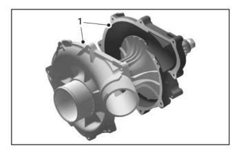
Inspect and clean supplied RIVA Impeller thoroughly taking care not to damage fins. Warm impeller using a heat gun or hair dryer. **NOTE: Do not use a torch.**
