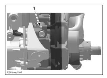
Remove supercharger unit from engine. **NOTE:** It is extremely important that the area utilized to work on the supercharger unit is very clean. Any foreign debris introduced into the supercharger unit will cause damage. It is equally important that care is taken when performing the following steps so as not to damage the impeller or working parts of the supercharger unit. Even a small mark on the impeller would ruin the dynamic balance causing severe damage.
