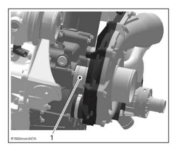
Install supercharger unit onto engine. NOTE: You may need to rotate supercharger impeller to allow supercharger gear to mesh with flywheel gear.
