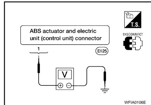
2. Check resistance between ABS actuator and electric unit (control unit) connector E125 and ground.
