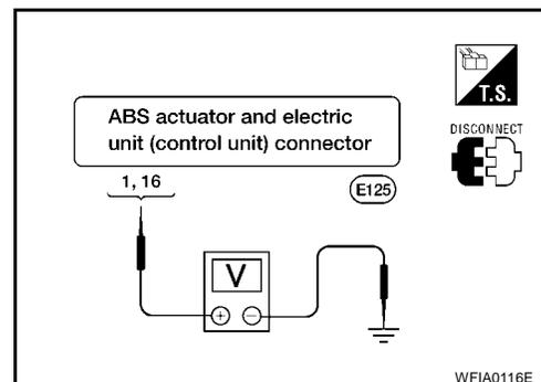
**3. CHECK ABS ACTUATOR AND ELECTRIC UNIT (CONTROL UNIT) GROUND CIRCUIT**
