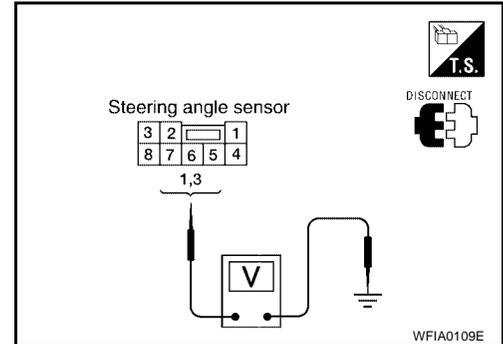
3. Check resistance between steering angle sensor connector M47 and ground.
