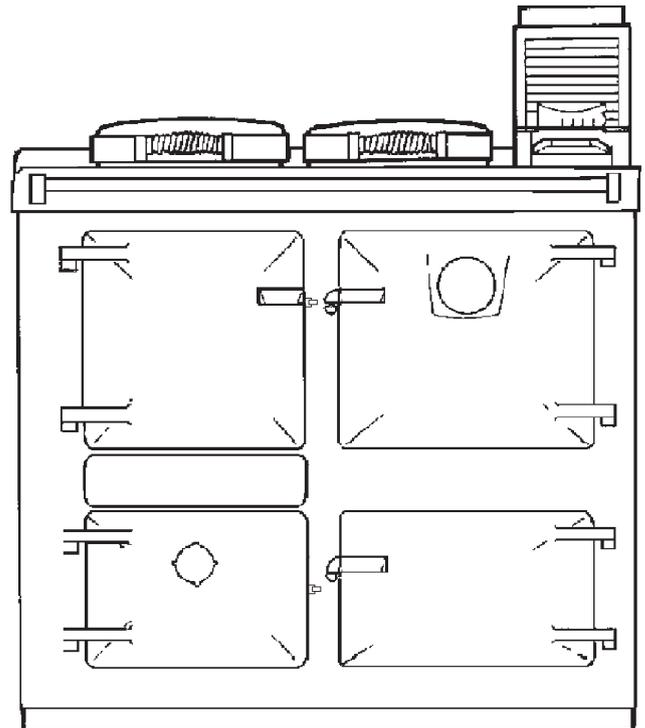
The temperature registered by the oven door thermometer may not necessarily correspond with the reading taken with a thermometer inside the oven
