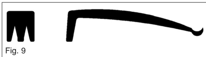
To open the doors. Use the utensil provided to turn the door release screw 1/4 turn counter-clockwise.
