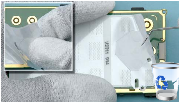
33) Release the DOMESHEET with the dental tool and peel it off. The DOMESHEET cannot be reused.
