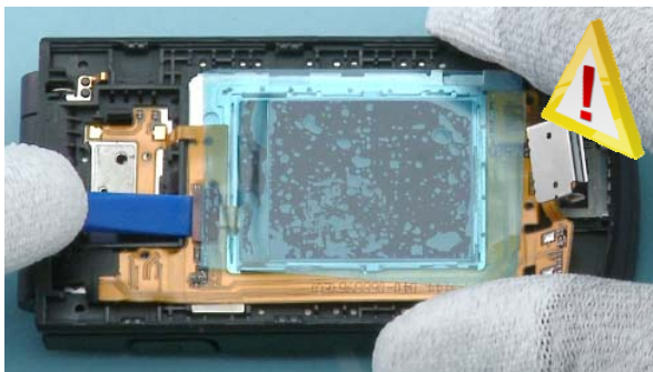
17) Disconnect the LCD connector with the SS-93. Be careful with the components around the connector!
