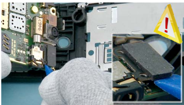
29) Before the engine board can be removed, the UI connector has to be disconnected from the engine board. Be careful with the components around the connector!
