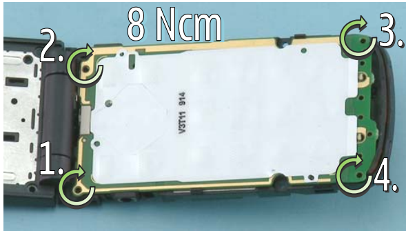
1) Tighten the four TORX + size 4 screws to the torque of 8 Ncm in the order shown.
