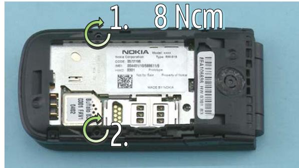
2) Tighten the two TORX + size 4 screws to the torque of 8 Ncm in the order shown.
