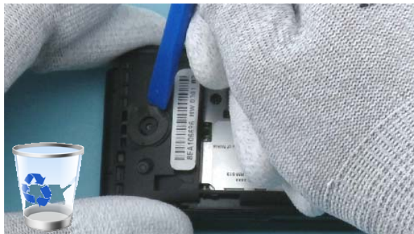
4) Use the SS-93 to release the CAMERA GASKET and remove it with the tweezers. The CAMERA GASKET cannot be used again.
