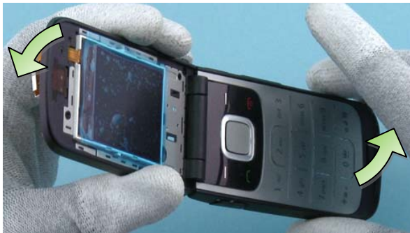
21) Flip the device carefully so that the LCD does not fall off!
