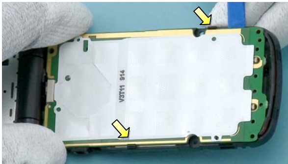
27) Carefully release the two clips holding the engine board with the SS-93.
