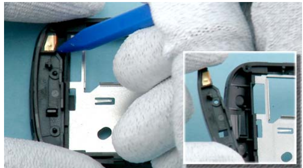
34) Use the sharp end of the SS-93 to detach the ANTENNA and then remove it.
