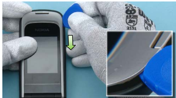
6) Open the phone and insert the SRT-6 between the IMD WINDOW and the B-COVER. Slide the SRT-6 along the window edges to loosen the adhesive.
