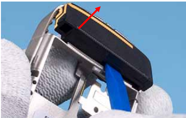
39.) Lift up the ANTENNA ASSEMBLY with SS-93 and remove it carefully.
