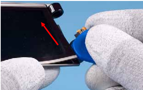
15.) Slide along the sides with SRT-6...
