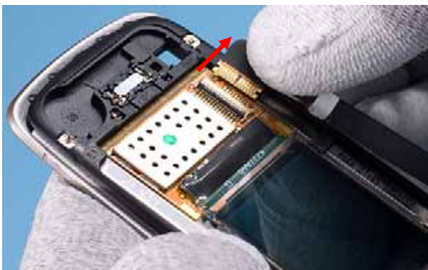
23.) Disconnect and remove the TOP FLEX.
