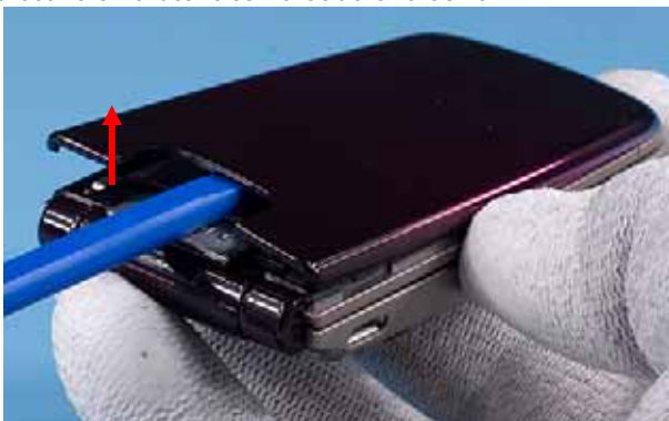
5.) Lift up the A-COVER carefully with SS-93. Pay attention to the display under the A-COVER.
