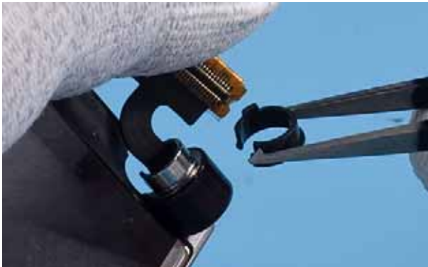
13.) Remove the HINGE WASHER with tweezers.
