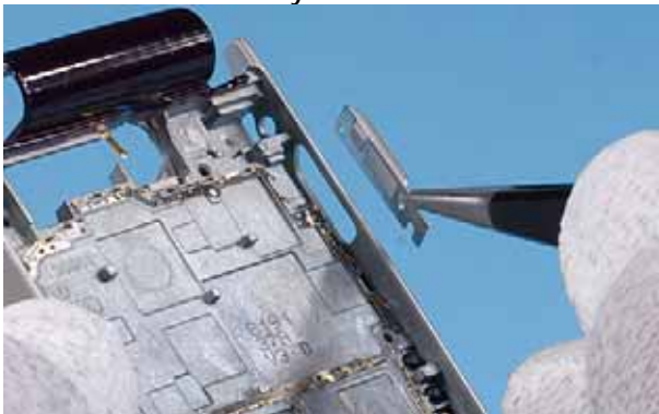
41.) Remove the OPEN KEY with tweezers.
