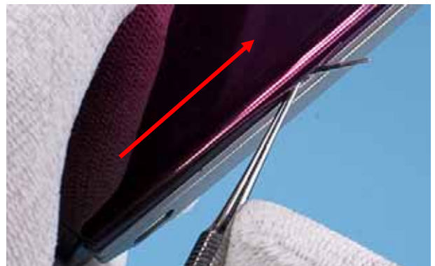
4.) Release the cover by sliding with the dental tool along the sides as shown in this picture.
