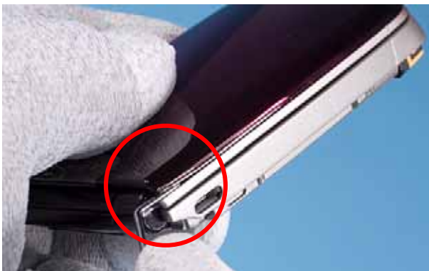
3.) Detach the A-COVER ASSEMBLY as shown in the picture and start to release the cover.
