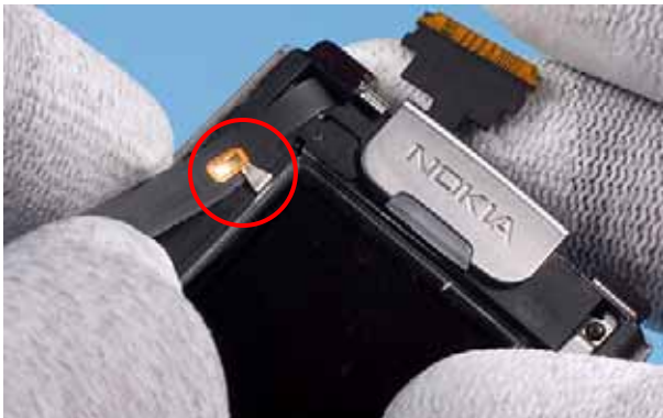
21.) Detach the TOP FLEX from the clip as shown.
