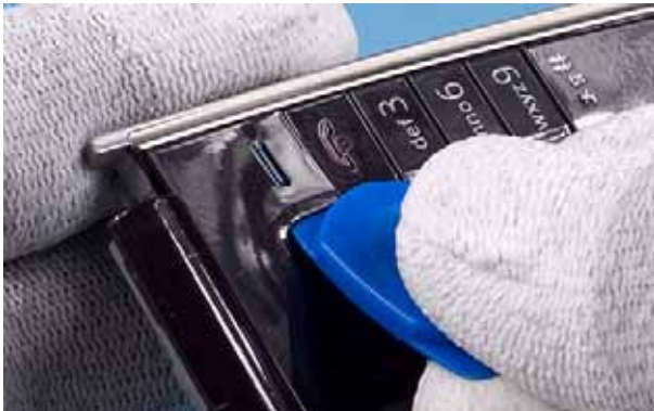
25.) Use the SRT-6 to open the KEYMAT KEY.
