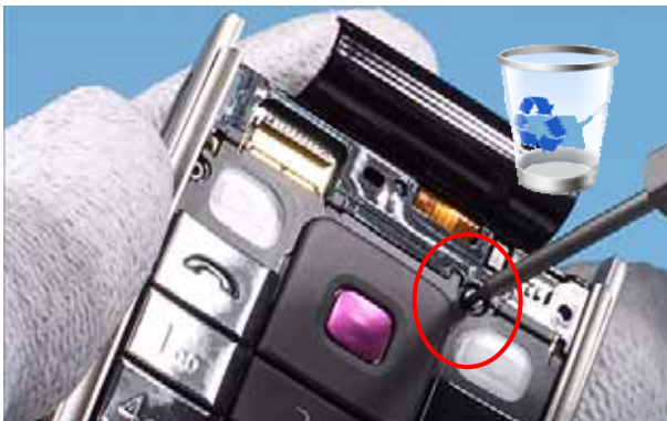
27.) Open the screw with SS-152 (SCREW BIT TX2IP).
