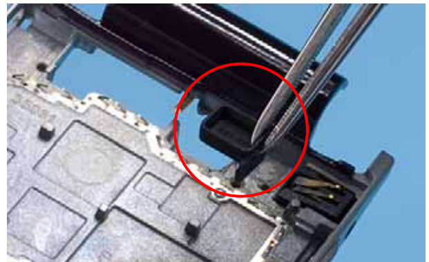
36.) Remove the MICROPHONE GASKET with tweezers.
