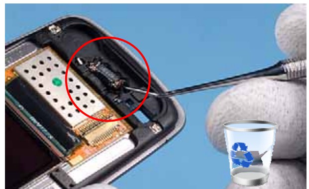
24.) Use the dental tool to remove the EARPIECE.
