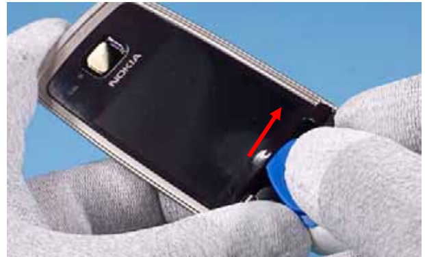
14.) Start to detach the DISPLAY WINDOW with SRT-6 carefully as shown in picture.
