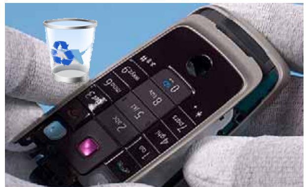
30.) ... until the KEYMAT can be removed easily.
