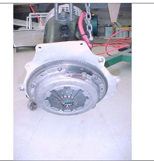
**Step 6:** Place the flywheel onto the hub and using the original flywheel bolts, bolt the flywheel onto the hub. Make sure there is Locktite on the bolts. Tighten the bolts in cris-cross pattern and torque the bolts according to the service manual specification.
