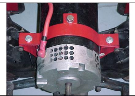
**Step 8:** Place the top motor mount over the motor and align the center hole with the lifting hole on the motor.
