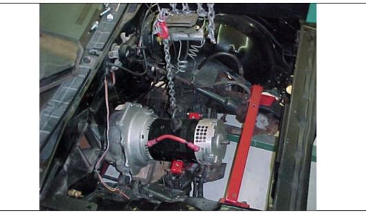
**Step 1:** Place the bottom half of the motor mount between the engine mounts and reuse the two original bolts removed with the engine to lock the motor mount in place.
