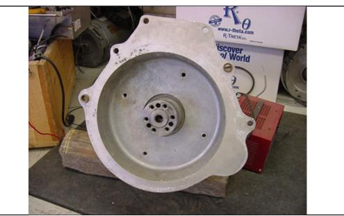
**Step 5:** Place the bell housing onto the motor and make sure the top of the bell housing is center with the lifting hole on the motor. Apply Locktite on the 3/8 x 1" bolts and tighten the bolts up.!!!!!!!IMPORTANT!!!!!!!!. Due to varying adapter thickness and motor type, your 3/8 bolts may be too long for your specific motor! After threading one bolt through the adapter and
