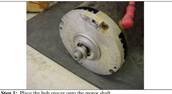
**Step 1:** Place the hub spacer onto the motor shaft
