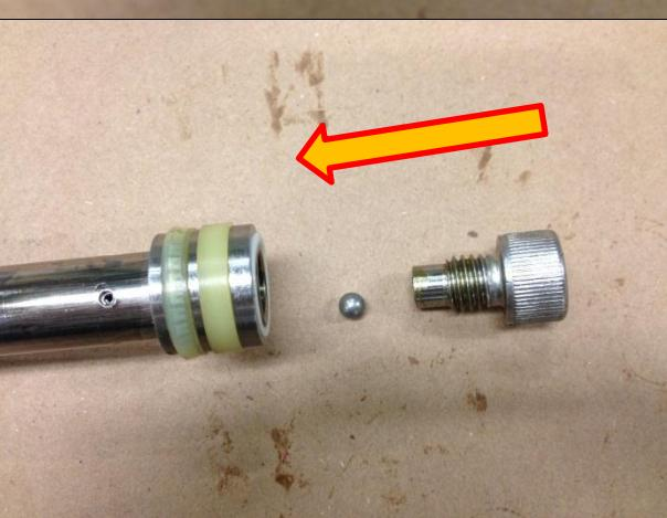
A photograph showing a piston assembly. A yellow arrow points from the text "Place the hub back on the piston, insert the ball and screw the valve seat on its place." to the hub of the piston. | Place the hub back on the piston, insert the ball and screw the valve seat on its place. |
