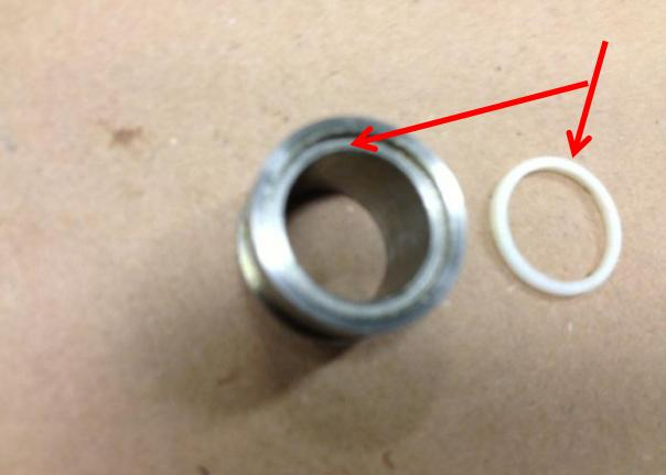
A photograph showing a metal hub and a white O-ring. A red arrow points from the text "Place the packing on the hub." to the O-ring.                                                               | Place the packing on the hub.                                                            |
