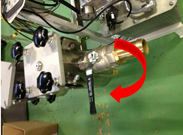
A photograph showing a close-up of a mechanical assembly with several valves and hoses. A red arrow points to a vertical handle valve, indicating the action to be performed.   | Close inlet valve to both glue- and hardener filter                                                                                                  |
