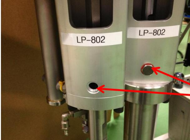
A photograph showing two vertical metal oil reservoirs labeled "LP-802". Two red arrows point to circular access ports or locks on the side of each reservoir.                 | Unscrew the locks of the oil reservoirs on top of the pumps and catch-up the oil (LP-802) from the reservoirs in a bucket.                           |
