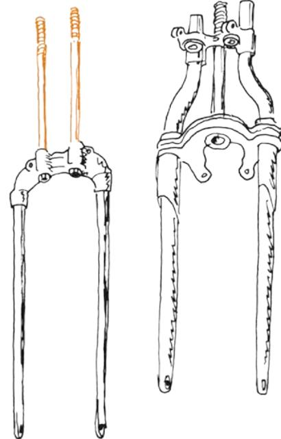
hole on the spring fork. The shock absorber rods must protrude from the fork by equal lengths.
