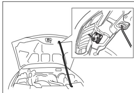
4. Before closing the engine hood, press the support rod firmly into its clip to prevent it from rattling.
