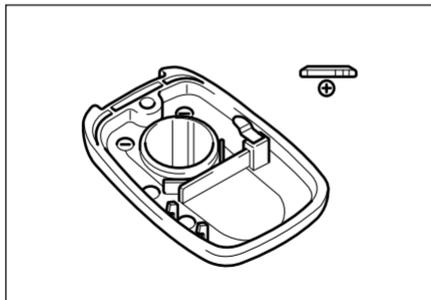
3. Fit the new battery, ensuring that correct polarity is maintained (positive (+) side facing down towards the base). Finger marks will adversely affect battery life ; if possible, avoid touching the flat surfaces of the battery and wipe them clean before fitting.
