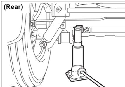
9. Remove wheel nuts completely by turning counterclockwise.
