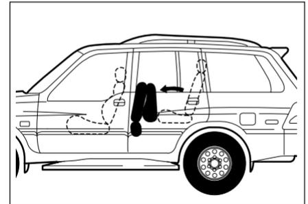
8. Make sure the seat belts are not twisted or caught in the seatback and are arranged in their proper position.
