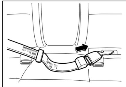
The buckle and metal latch plate of the center rear lap belt are identified by the "CENTRE" mark. Be sure to check the marking before wearing the center rear lap belt.
