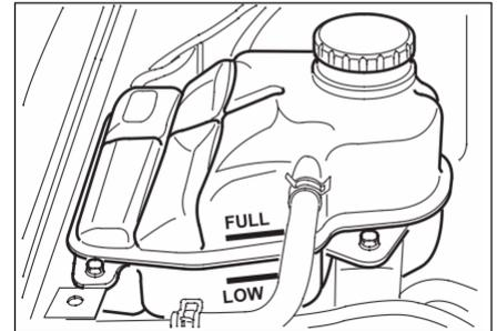
In order to protect your vehicle in extremely cold weather, use a mix 40% soft water and 60% antifreeze specified.
