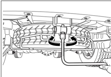
1. Rotate the latch bolt counterclockwise as shown using the wheel nut wrench.
