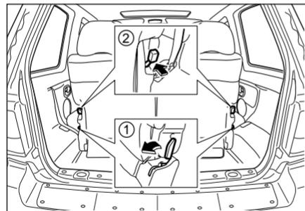
4. Make sure the seat erect with pushing the levers ③ from the right to the left.
