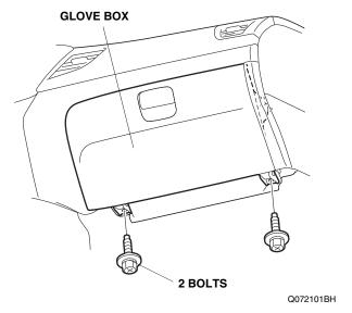
• Open the glove box, push inward on the stops, and remove the glove box.
