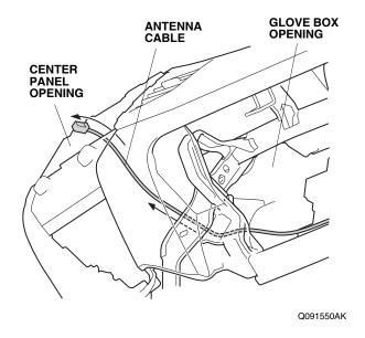
41. Route the antenna cable through the center panel opening, and align it with the vehicle connector.
