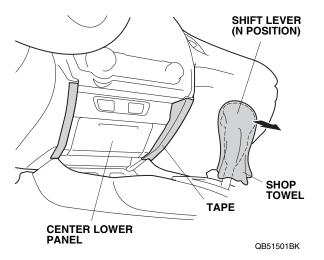
Remove the center lower panel (two self-tapping screws, four clips, and unplug the vehicle connectors, if equipped).
