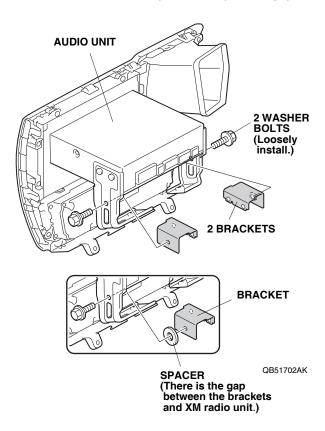
Install the XM radio unit to the brackets in the audio unit with four washer bolts.
