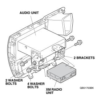
24. Secure two washer bolts installed in step 22.
