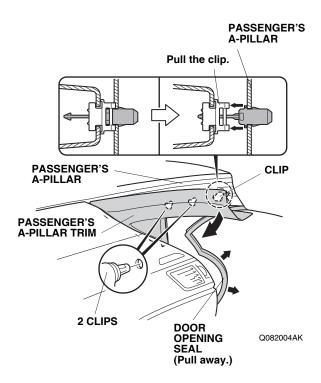
Pull out the passenger's A-pillar trim to release the clips.
