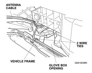
46. Cut one urethane tape, and wrap the piece of urethane tape around the antenna cable as shown.
