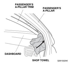
11. Remove the passenger's A-pillar trim from the upper clip (unplug the vehicle connector, if equipped). Carefully remove the shop towel and any clips that fell from the passenger's A-pillar trim.
