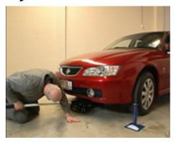
Roll the jack under the vehicle, and make sure the pad, or saddle, is positioned correctly under the frame or cross member.
