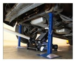
Use the jack to raise the vehicle off the safety stands. Slide out the safety stands from under the vehicle.
