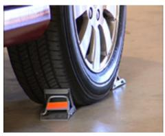
Double check the position of the wheel blocks to make sure they haven't moved.
