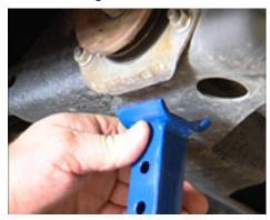
Slide the two jack safety stands underneath the vehicle. Make sure they're positioned at a point that can support the weight.
