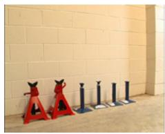
Before operating the jack, select two safety stands of the same type, suitable for the weight of the vehicle.
