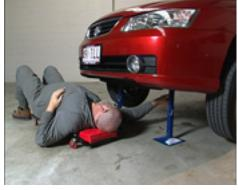
When you've finished working under the vehicle, make sure you've removed all tools and equipment before you attempt to lower it.
