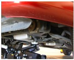
Turn the valve on the jack handle counter-clockwise very gently to lower the vehicle to the ground. Do not allow the vehicle to drop quickly or you may cause serious damage.
