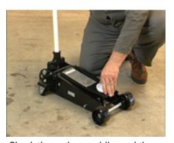
Check the pad, or saddle, and the wheels of the jack. They should rotate freely and show no signs of damage.
