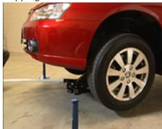
If the vehicle is stable, continue lifting it until it's at the height where you can safely work under it.
