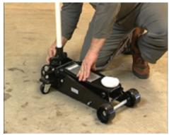
Before you try to use the jack, check for leaks in the hydraulic system.
