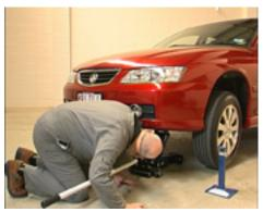
Once the wheels lift off the floor, stop and check the placement of the jack pad under the vehicle to make sure there's no danger of slipping.
