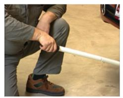
Turn the valve on the jack handle counter-clockwise and gently lower the vehicle onto the stands.
