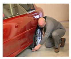
Then place blocks in front of and behind the wheels that aren't going to be raised off the ground.
