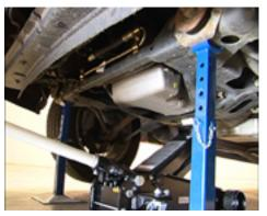
When the vehicle has settled onto the stands, lower the jack completely and remove it from under the vehicle.
