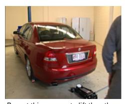
Repeat this process to lift the other end of the vehicle. Be aware that the vehicle is now supported on jack stands and will not be as stable as it would if the wheels were on the ground.
