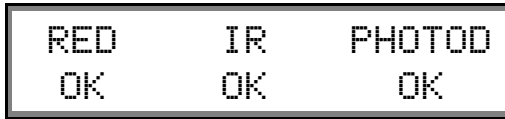
Figure 2 - Red LED (RED), infrared LED (IR), and photodiode (PHOTOD) circuits of sensor functional ("OK").
