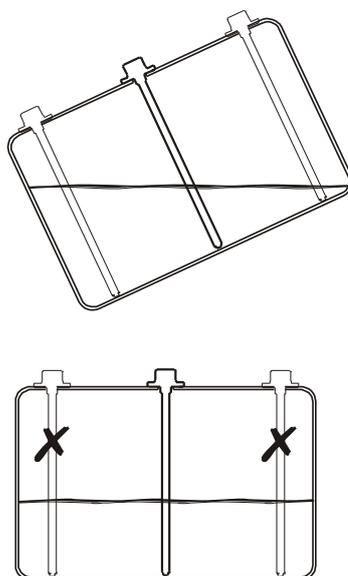
*Pic. 8.1 Proper position of sensor on fuel tank*
