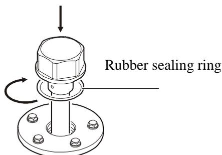
*Pic. 8.7 Installation of assembled sensor on fuel tank*
