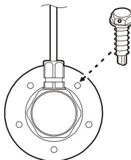
*Pic. 8.3 Position of screw with a hole for sealing*
