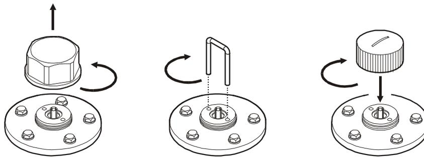
*Pic. 10.1 Partial removal of fuel level sensor*
