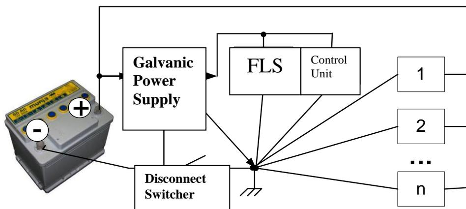
Pic. 8.11 Installation of sensor on vehicle if it is necessary to save functionality when "mass" is switched off.
