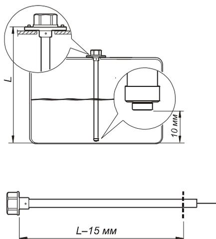
*Pic. 8.4 Determining of measuring probe's length*
