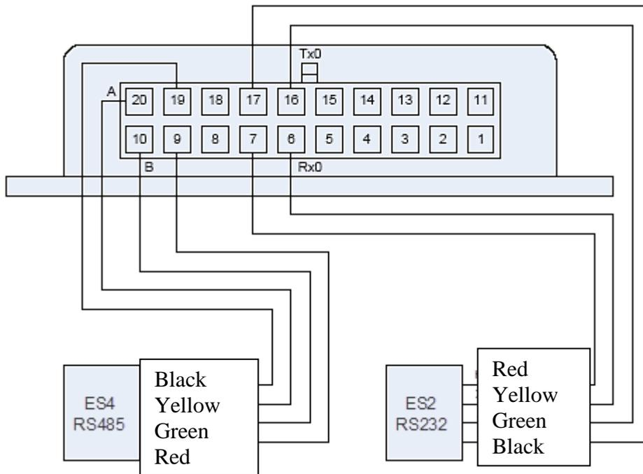
*Pic. A4.2. Connection of sensors with different interfaces RS485+RS232*
