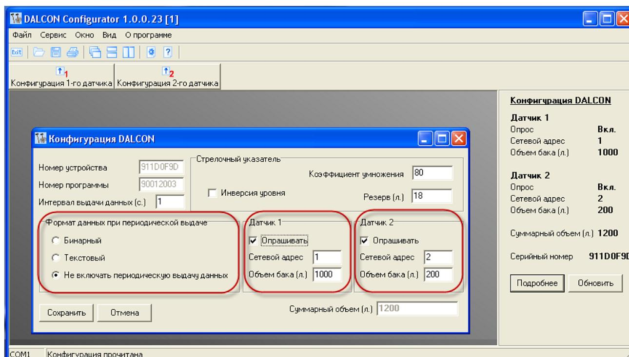
Pic A4.5. Typical DALCON configuration for devices using a digital protocol.
