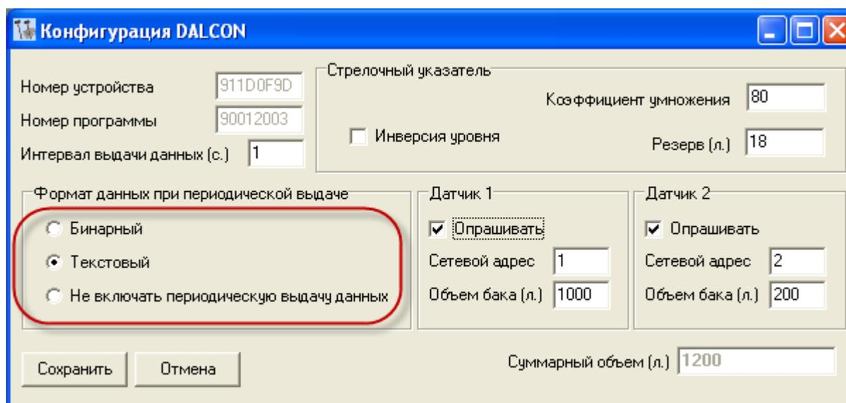
*Pic. A4.6. A typical DALCON configuration for devices using a text protocol*
