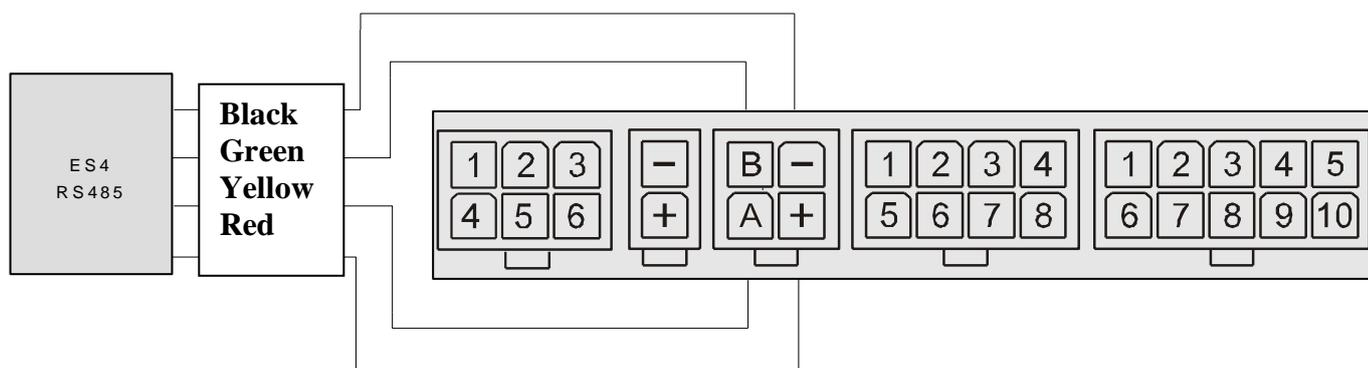
Depending on your sensors board that are part of the system Teletrack to the control unit 1 or 2 FLS can be connected, with the capacity of 10 or 12 bits.
