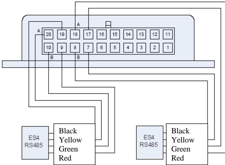
*Pic. A4.1. Connection of sensors with the same interfaces RS485.*
