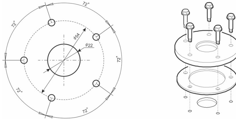
*Pic. 8.2 Size and method of flange setting on fuel tank*
