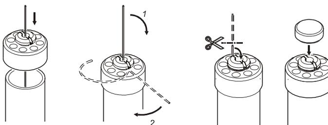
*Pic. 8.5 Method of fastening of string on the end of probe*
