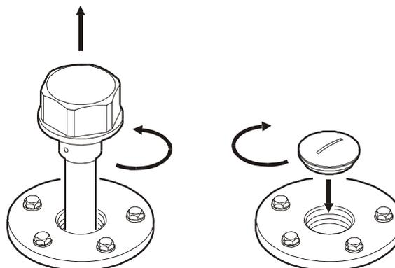
*Pic. 10.2 Complete removal of fuel level sensor*
