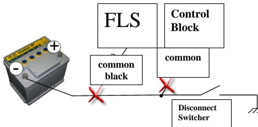
Pic. 8.10 INCORRECT connection of common wire.
