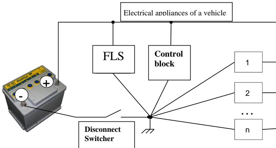
*Pic. 8.9 CORRECT connection of common wire*
