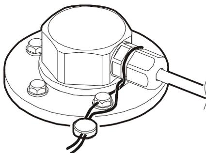
*Pic. 8.12 Method of sealing of the installed fuel level sensor*
