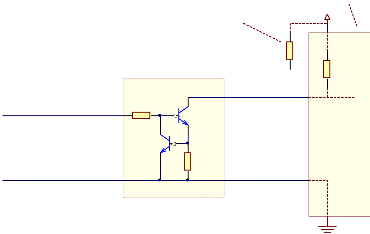
*Diagram of the matching device to match the frequency output from the frequency of FLS and input device of vehicle monitoring (output - open collector, the maximum load current - 25 mA).*
