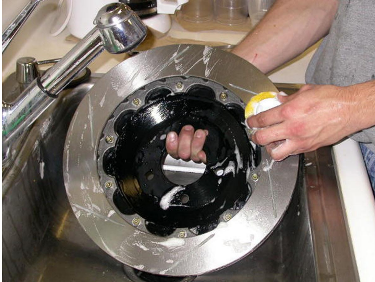
Scrubbing the rotor with a Scotch-brite pad in soap and water
