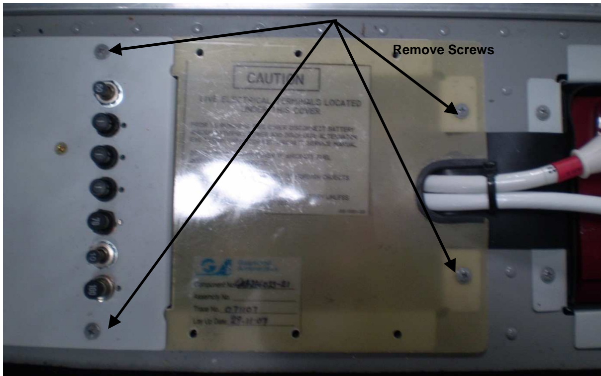
Figure 1 : Screws to be removed to gain access to internal assembly of the solenoid box
