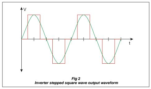
This is important for circuits where magnetic devices, such as transformers and contactors (RMS voltage) are in circuit with electronic relays that derive their DC voltage from capacitor input filters (peak voltage).
