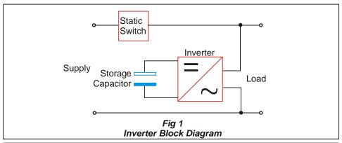
The STATIC SWITCH is robust and can withstand large current surges. It is ideally suited for contactor operation where high peak currents of short duration occur during energizing.
