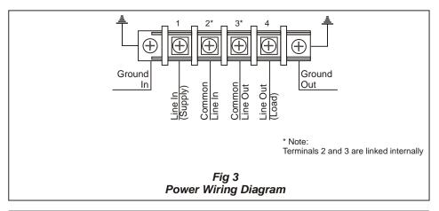
9. Once the unit has been mounted and the external wiring completed, power can be applied. Turn on the power to the unit. After about two seconds the green LED indicator "System OK" should come on. The unit is now fully operational.
