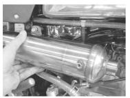
3 . After inserting the exhaust pipe into the joint on the canister assembly, insert its flange into the engine
