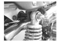
6 . Tighten the exhaust pipe flange nuts evenly to the specified torque with care not to let the canister and the exhaust pipe get out of the adjusted places.
