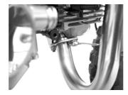
. Next, tighten the flange bolt on the canister bracket to the specified torque.
