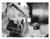
3 . Unfasten the nut on the back side of the exhaust system.
