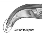
4 . If the exposing portion is cut off, it is advisable to give a touch-up to the cut surface with a heat-resistant paint to prevent the surface from rusting.
