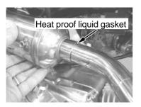
It is advisable to apply heat-resistant liquid gasket to the inserting portion. (ThreeBond 1207B or the equivalent.)
