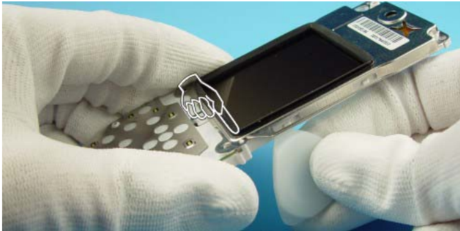
Open the shield snaps on both sides with SRT-6.
