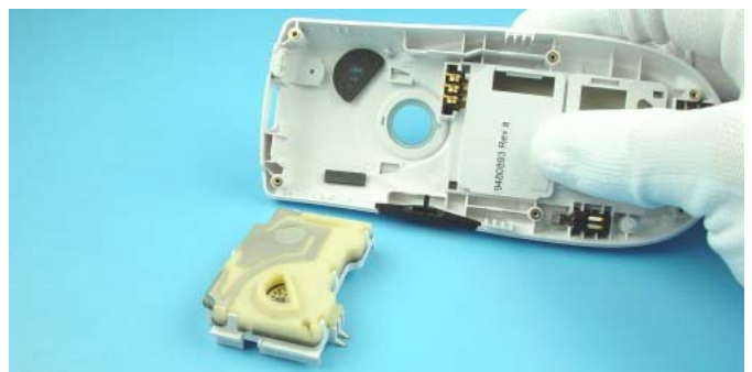
Antenna drops out when turning B-Cover.
