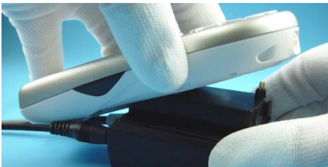
Insert the Flash Adapter FLA-48 like a battery, start at the battery connector site.
