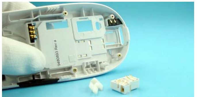
Turn B-Cover let System Connector with Connector Retainer drop out.
