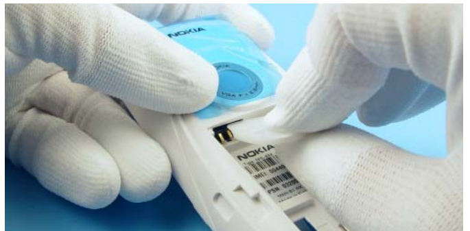
To remove the Battery Connector, use SRT-6 Opening Tool.
