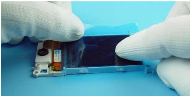
Always protect LCD with protection foil to avoid dust and scratches.
