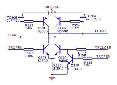
Figure 3.2.4.1 Open/close door circuit diagram
