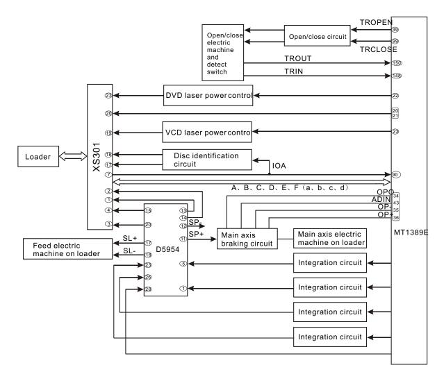
Figure 3.2.2.1 Servo circuit block diagram
