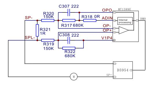
Figure 3.2.6.2 Main axis braking control equivalent circuit diagram
