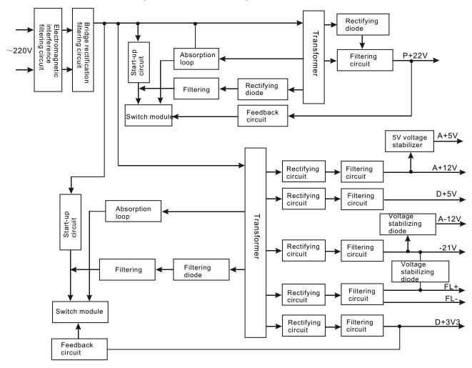
Figure 3.2.12.1 Power circuit block diagram
