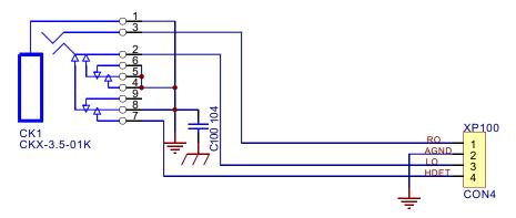
Figure 3.2.8.3 Headphone board schematic diagram
