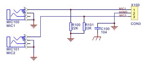
Figure 3.2.8.2 MIC board schematic diagram
