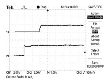
2. Waveform diagram of the comparison between power-on mute signal (channel 1) and +12V (channel 2) power supply:
