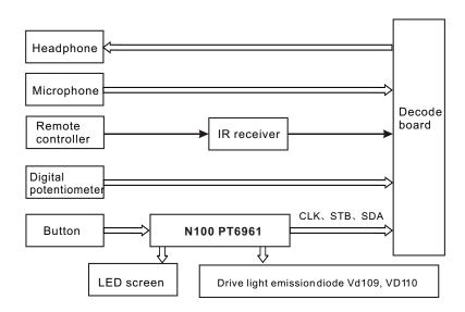
Figure 3.2.8.1 Panel control components block diagram
