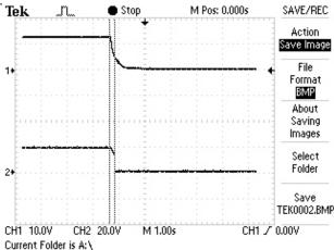
4. Waveform diagram of the comparison between LRSWM signal (channel 2) and +12 power (channel 1) when power on. The increase of LRSWM signal goes through 2 steps: the first is 0.6V with durable time 6.5 S; the second is 16V with duration time 13.5 S.
