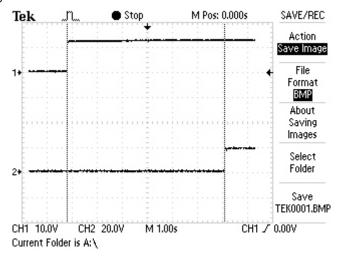
3. Waveform diagram of the comparison between HARDM signal (channel 2) and +12V power (channel 1) when power off:
