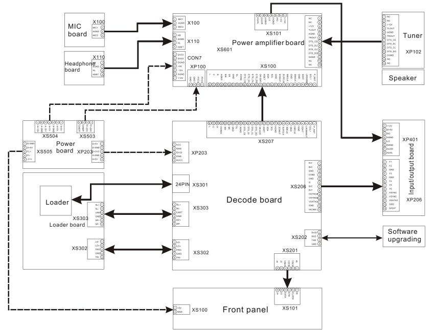
Figure 3.1.2.1PC Bboard block diagram of the player
