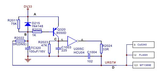
Figure 3.2.5.1 Reset circuit diagram
