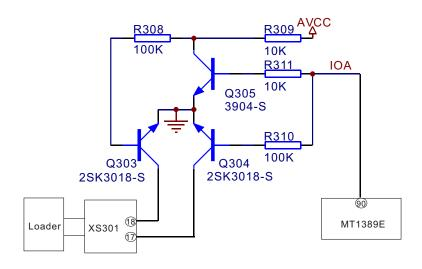
Figure 3.2.7.1 Disc identification circuit
