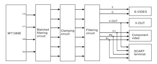
Figure 3.2.9.1 Video circuit block diagram
