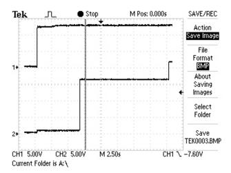
5. Waveform diagram of the comparison between LRSWM signal (channel 1) and LRSWMUT signal (channel 2). When mute is on, 1389 gives out low level signal LRSWMUT mote than 310ms to make LRSWM signal level pull down to make mute output, and 1389 is mute from inside to make all channels have no output. Centre, surrond channel mute means is the same with that of main channel.
