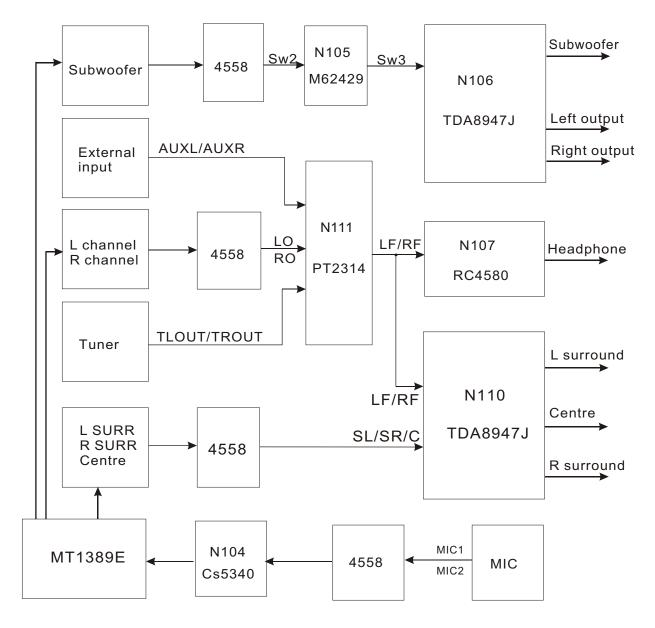
Figure 3.2.11.1 Audio power amplifying circuit diagram
