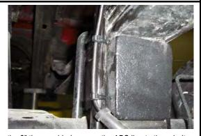
Using the 8" ties provided, secure the ABS line to the u-bolt.
