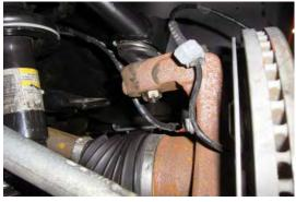
Tighten the three upper strut mounting nuts to 45 ft-lb. Install the upper ball joint to the knuckle. Tighten to 85 ft-lb. Install the supplied cotter pin.
