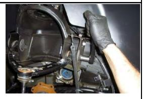
Mark the position of the alignment cams. Remove the 21mm UCA nuts, cams, and bolts.
