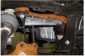
Install the driver side differential drop bracket using the M12x40 and M12x45 socket cap bolts. Tighten to 75ft-lb (4WD Only)
