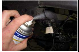
Lubricate the ABS line with WD-40 and slide the rubber sleeve up to allow the wire to be reinstalled in the clip on the frame.
