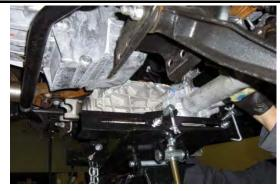
Raise the differential back up into its mounting location. Take care not to pinch the electrical line. (4WD Only)
