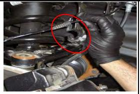
Unclip the ABS line at the upper control arm and unbolt the brake line retention bracket on both sides
