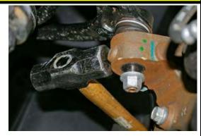
Separate the upper ball joint from the steering knuckle. Repeat on opposite side.
