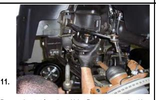
Remove the strut from the vehicle. Repeat on opposite side.
