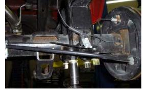
Install the new u-bolts, factory axle plate, washers, and nuts provided. Tighten to 136lb-ft.
