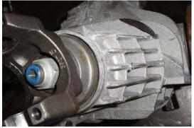
Use a black permanent marker to mark the material to be removed. This will be on the driver side of the differential. (4WD Only)
