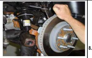
Remove the six 15mm axle shaft bolts. Set the hardware aside as it will be reused. Repeat on opposite side. (4WD Only)
