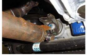
Set the straps and bolts aside. Slide the driveshaft back off the yoke. (4WD Only)
