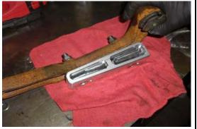
Bolt the 2" wide diff drop bracket (narrow taper facing the rear) to the torque arm using the M12x70 and M12x80 socket cap bolts and M12 flange nuts. 75ft-lb. (4WD Only)
