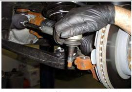
Unbolt the tie rod end using a 21mm socket. A additional wrench may be need to keep the ball joint from spinning. Repeat on opposite side.
