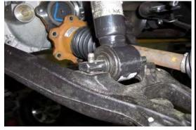
Raise the lower control arm and line up the lower mounts. Install the M10x55 bolts, washers, and nyloc nuts. Tighten to 45 ft-lb.
