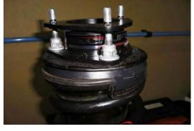
Install the ReadyLift Strut Extension on top of the strut using the factory hardware. Tighten to 45 lb-ft.
