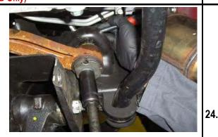
Remove the passenger side torque arm using a 15mm socket and 18mm socket. (4WD Only)
