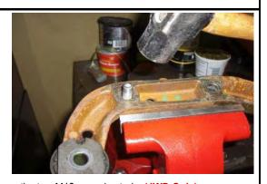
Remove the two M12 press in studs. (4WD Only)
