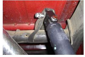
Install the shock extension into the upper mount using the factory bolt. Do not tighten.
