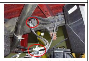
You may need to bend the upper and lower brake line brackets to allow enough slack in the line at full droop.
