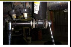
Install the shock into the lower mount using the factory hardware Tighten to 136 lb-ft.
