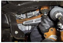
Reinstall the torque arm to the frame mount. Torque the factory hardware to 75ft-lb. (4WD Only)
