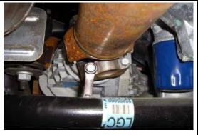
Remove the four 11mm driveshaft bolts. (4WD Only)
