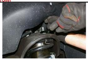
Remove the three 18mm upper strut mounting nuts.
