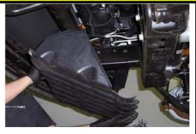
Remove the front wheels. Unbolt the five 15mm bolts that hold the plastic air dam on. Set aside.
