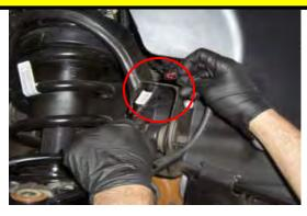
Unclip the ABS line at the upper control arm pocket on both sides.
