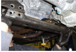
Put the cross member back in place. Use of a rubber mallet may be needed to help persuade the cross member mounting holes to line up. (4WD Only)
