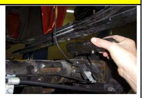
Lower the axle and remove the factory block.
