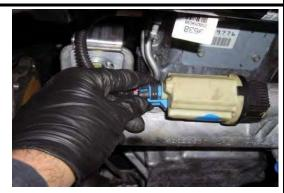
Reconnect the tabs from the wiring harness and plug the connector back in. (4WD Only)
