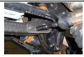
Remove the four rear cross member nuts and bolts. (4WD Only)
