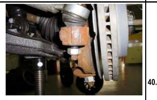
Re-install the tie rod. Tighten to 118 ft-lb.
