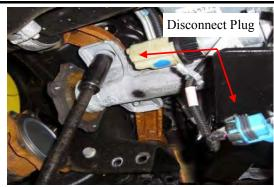
Disconnect the blue electrical plug from the front differential. Support the front differential with a transmission jack. Remove the two passenger side mounting nuts. (4WD Only)
