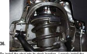
Re-install the strut into its stock location. Loosely install the M10 flange nuts on the upper mount.
