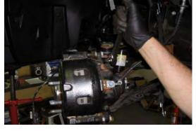
Install the front brake calipers using the factory hardware and 18mm socket. Tighten to 146 lb-ft.
