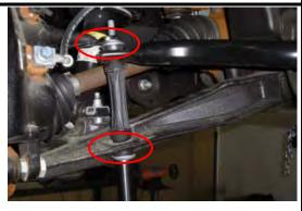
Remove the sway bar end link bolt using a 15mm socket and a 15mm open end wrench. Do this on both sides
