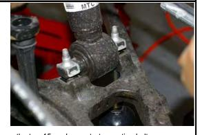
.Remove the two 15mm lower strut mounting bolts.
