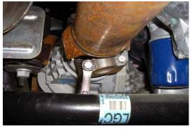
Re-install the front driveshaft using the factory hardware and clamps. Tighten to 26 ft-lb. (4WD Only)
