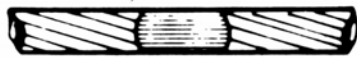
Example of properly fused weld nugget (approximate solid area of two times diameter of conductor).
