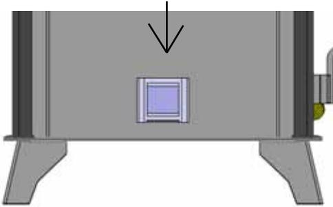
The shaker handle bolts onto the shaker block using the bolts and lock washers provided.
