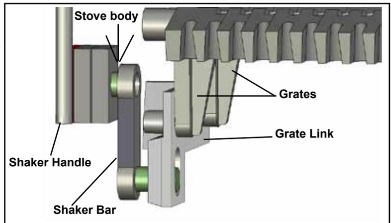
Your grates will last forever, as long as you keep your ashes cleaned out of the stove. When ashes are left pile-up against the grates, the air-flow is blocked. With no air flow through the grates, they will begin to sag from the intense heat.
