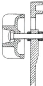
The viewing glass is installed between the door and the window frame. The glass gasket is installed only on the sides of the glass panel. The top and bottom of the glass are open to provide air-wash and secondary air to the firebox. The glass frame is secured to the door with four bolts.
