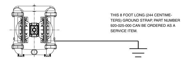
To reduce the risk of static electrical sparking, this pump must be grounded. Check the local electrical code for detailed grounding instruction and the type of equipment required, or in the absence of local codes, an industry or nationally recognized code having jurisdiction over specific installations.
