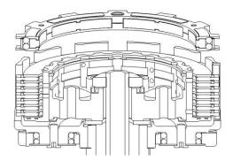
NOTE: Some OEM Baskets have "half slots" at the top of the basket tangs—with Rekluse products we require that all friction disks, including EXP disk, are seated into MAIN basket slots.
