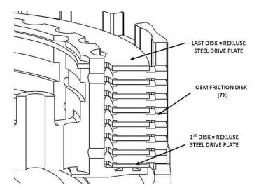
**NOTE:** Some models have a clutch boss spring in the OEM friction pack. This consists of two metal rings and one narrow friction disk. Do Not Re-install these with the Core EXP
