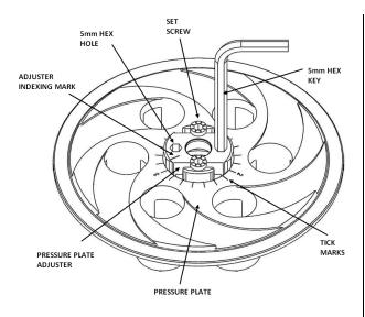
**NOTE:** The pressure plate comes with the set screws and adjuster installed. For reference, if the set screws are ever removed, the knurled side should face up.
