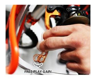
The following steps explain two ways to check Free Play Gain. One will use the rubber band that has been included in the clutch kit and one explains using your hand, which you will perform before every ride.
