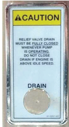
Figure 4-3: Intake Relief Valve Drain
