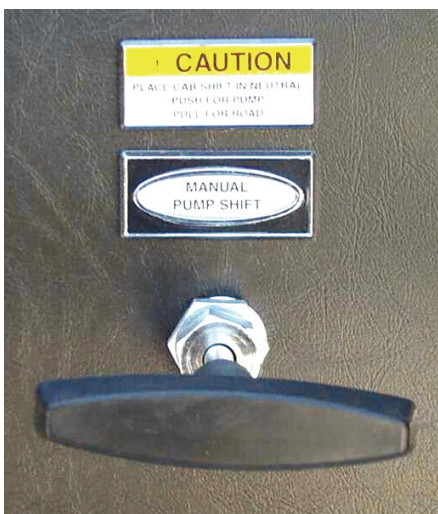
Figure 3-2: Manual Pump Shift Override
