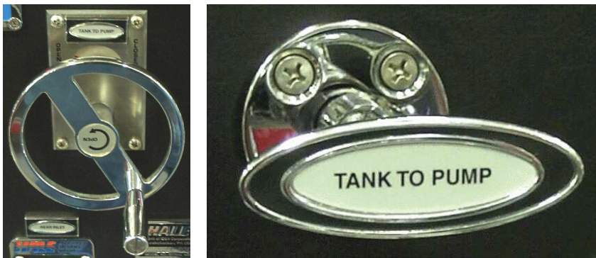
Figure 3-3: Typical Tank-to-Pump Valves
