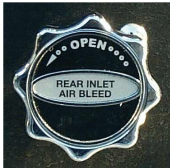
Figure 3-16: Air Bleed Valve
