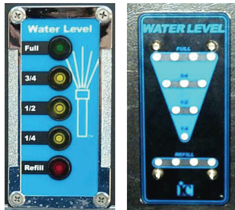
Figure 3-13: Typical Tank Level Indicators
