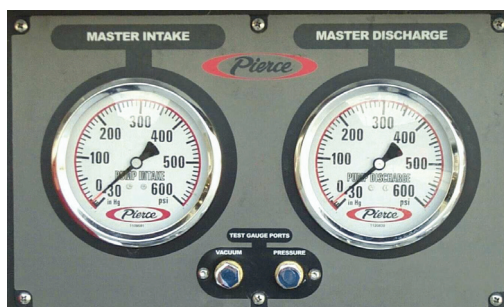
Figure 3-9: Master Discharge Pressure Gauge (Right)
