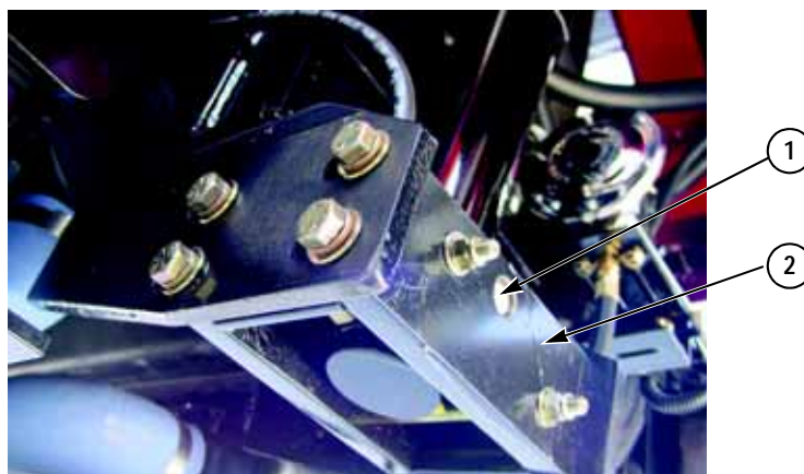
Figure 4-1: Typical Lift Cylinder Trunnion & Bracket
