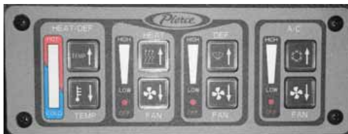
Figure 3-10: HVAC Control Panel
