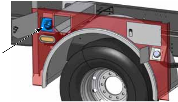
Figure 3-8: Typical DEF Reservoir Location
