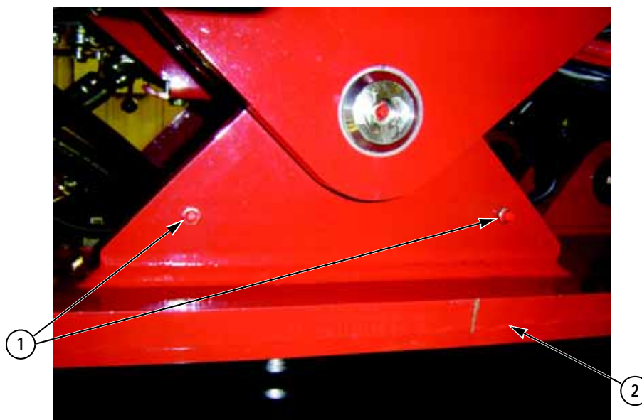
Figure 4-5: Fifth Wheel Bearing Grease Fittings
