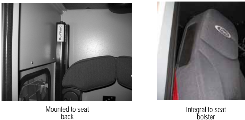
Figure 3-5: Inflatable Head Curtain (IHC)/Supplemental Restraint Air Bag (SRA)
