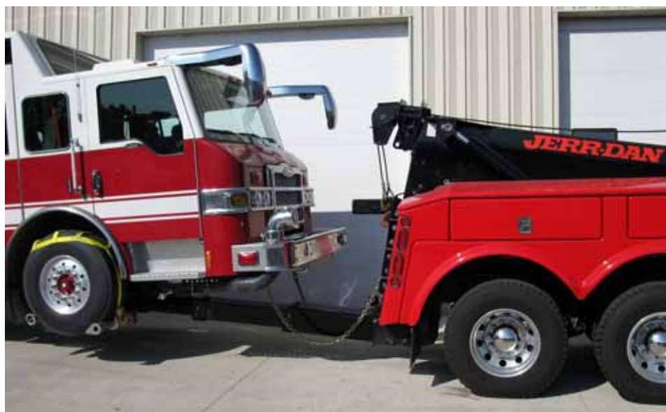
Figure 4-8: Underlift Device using Tire Lift Brackets
