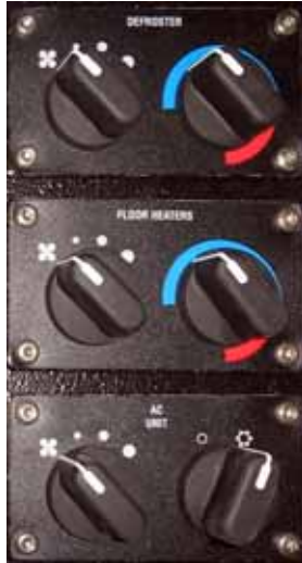
Figure 3-9: HVAC Control Panel
