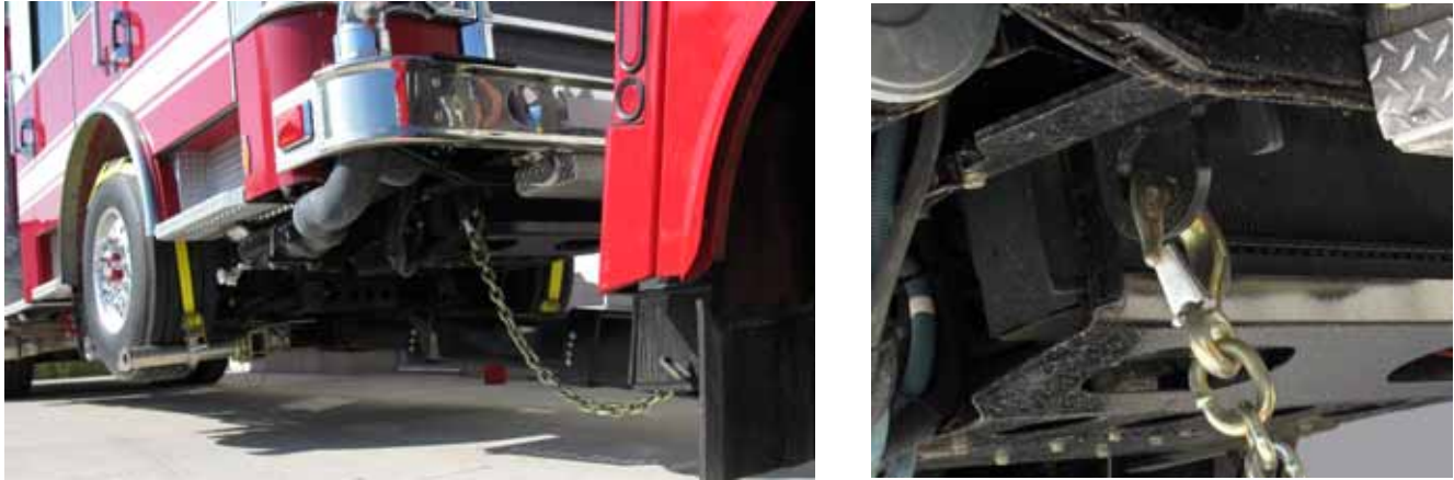
Figure 4-9: Safety Chains and Tire Straps
