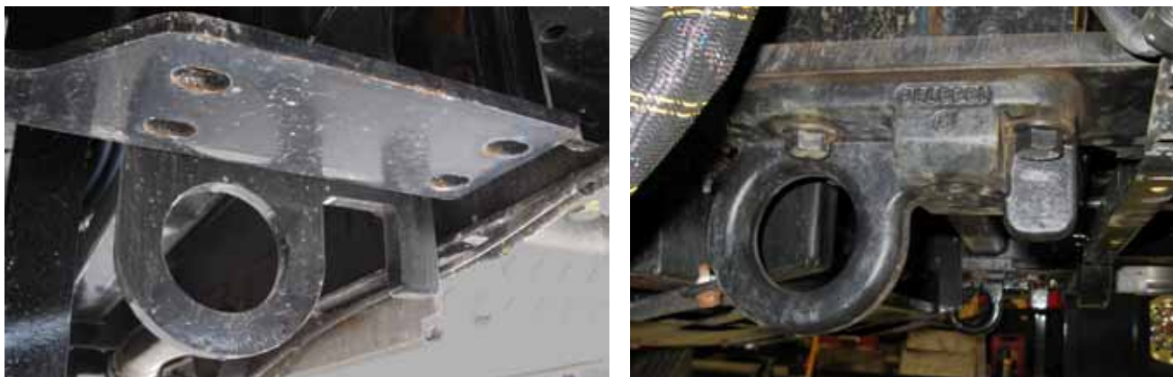
Figure 4-10: Lift and Tow Saddle Brackets with Integral Tow Eye
