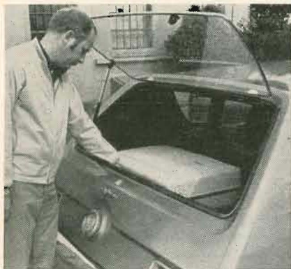
The rear window in our Gremlin opens for loading, but the liftover is quite high
