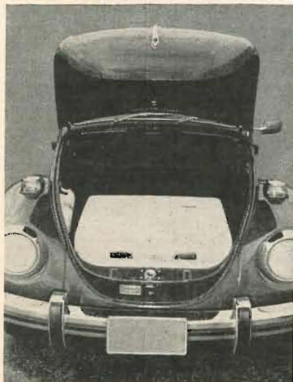
The Super Beetle 's trunk is much larger than the nonsuper VW 's, thanks to a new front suspension and a bulge in the hood
