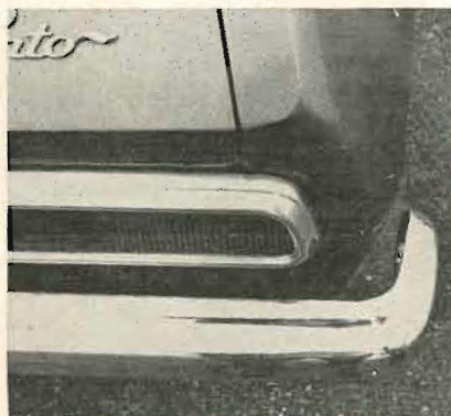
Unlike most small cars, the Pinto has space between its rear bumper and body metal; this helps prevent parking scars
