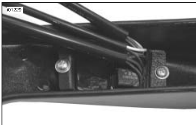
Figure 3. Turn Signal Unit Installed
