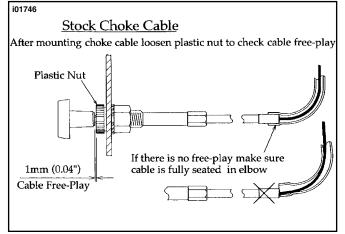
Figure 10. Proper Choke Cable Free Play
