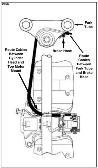
Figure 8. Throttle Cable Routing (XL Models)
