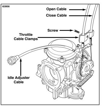
Figure 6. Throttle Cable Installation (Buell)
