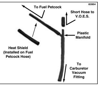
Figure 2. Original Vacuum Hose Configuration
