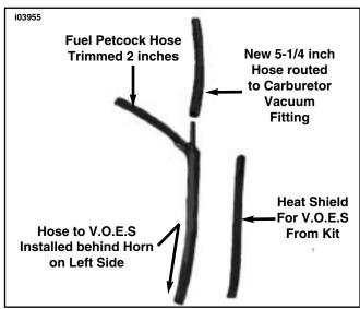
Figure 3. Modified Vacuum Hose Configuration
