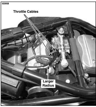
Figure 9. Throttle Cable Routing (Buell Models)
