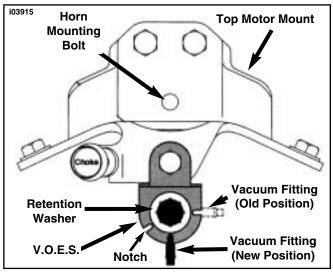
Figure 5. V.O.E.S. Installation
