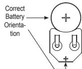
Battery replacement is 3 volt lithium coin cell type 2032.
