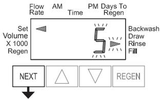
**Step 6CS** – Set duration of the special rinse cycle to be performed prior to a valve returning to Service. Selectable from 1 - 20 minutes or OFF. Only viewed if 2.0 is set in 2CS, and ALTA or ALTb is set in 5CS.
