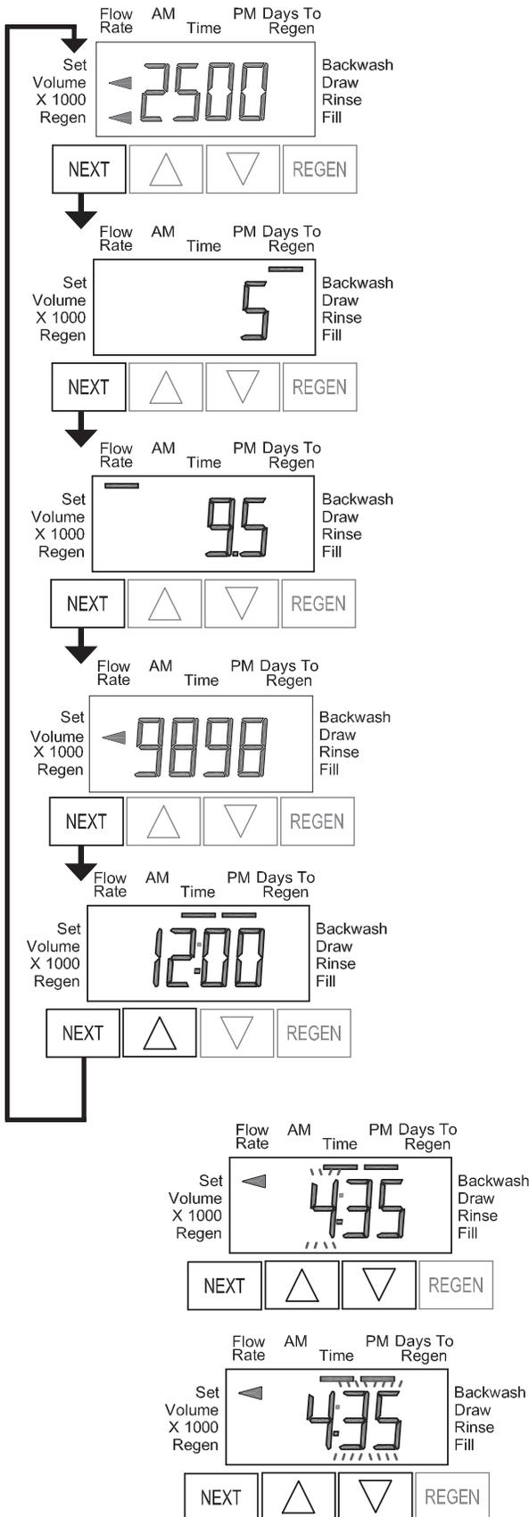
When the system is operating, one of five displays may be shown. Pressing NEXT will alternate between the displays shown below.
