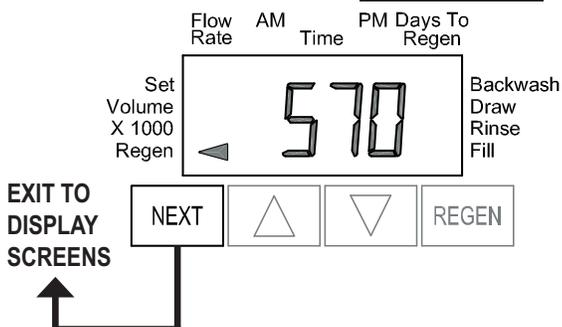
**Step 1D** - Press ▲ and ▼ buttons simultaneously for 5 seconds and release. Then press ▲ and ▼ buttons simultaneously for 2 seconds and release. If screen in Step 2D does not appear the lock on the valve is activated. To unlock press ▼, NEXT, REGEN, ▲ in sequence, then press ▲ and ▼ buttons simultaneously for 5 seconds and release. Then press ▲ and ▼ buttons simultaneously for 2 seconds and release.
