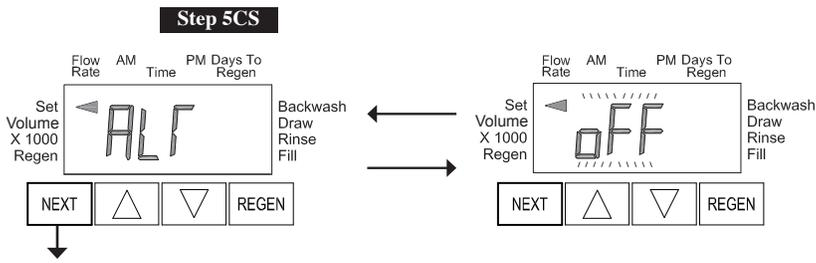
**Step 5CS** – Allows selection of one of the following using the ▲ or ▼ buttons:
