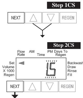
**Step 1CS** – Press ▲ and ▼ buttons simultaneously for 5 seconds and release. If screen in Step 2CS does not appear, the lock on the valve is activated. To unlock press ▼, NEXT, REGEN, ▲ in sequence, then press ▲ and ▼ buttons simultaneously for 5 seconds and release.
