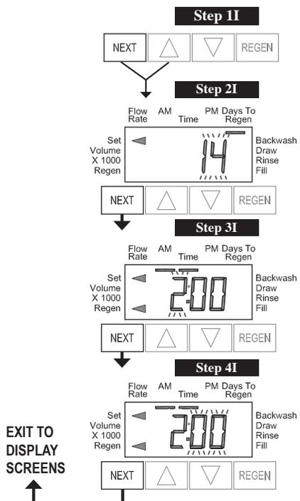
**Step 1I** - To enter Installer Display press the NEXT and ▲ buttons simultaneously for five seconds and release.
