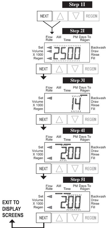
**Step 1I** - To enter Installer Display press the NEXT and ▲ buttons simultaneously for 5 seconds and release.
