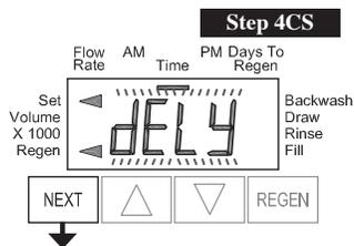
**Step 4CS** – Press the ▲ or ▼ buttons to select to regenerate immediately on 0 or at delayed time.
