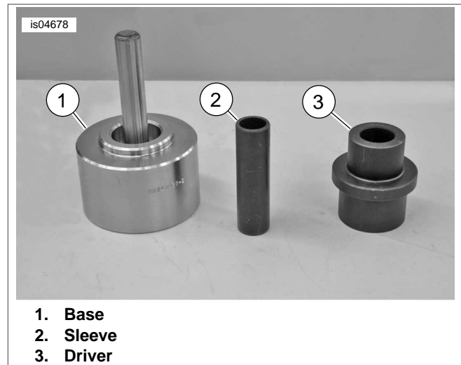
Figure 2. Rear Wheel Compensator Sprocket Bearing Remover/Installer (HD-48921)
