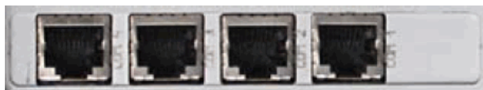
Figure 9. Serial ports on the MIB800 or MIB850.
