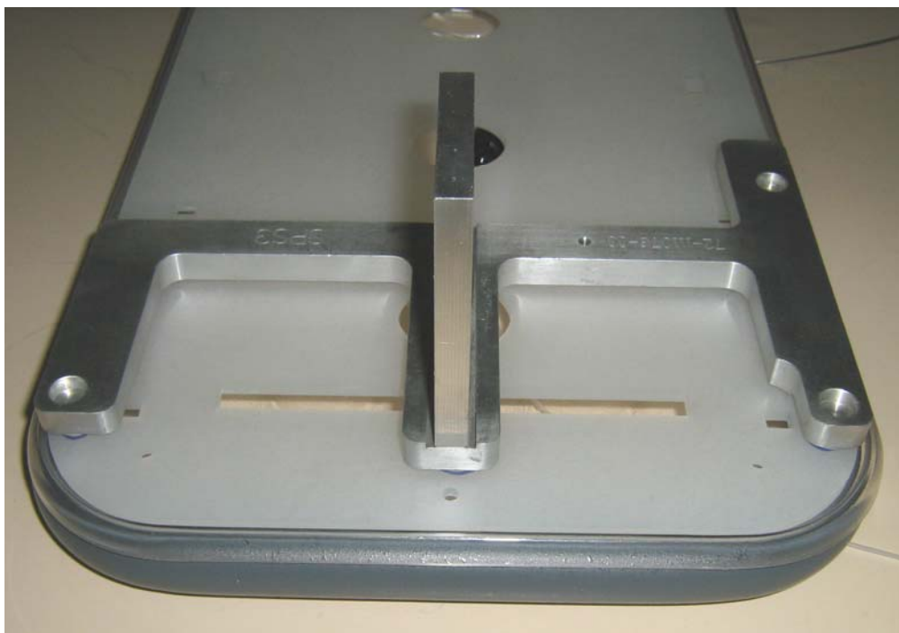
Figure 54. Alignment Tool Position in the Tray for B Point Calibration
