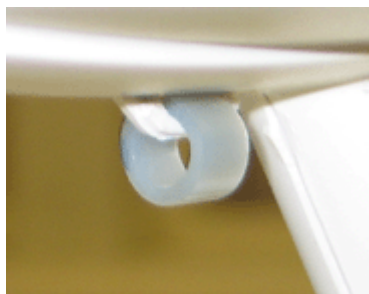
Figure 4. Retaining loop on underside of the probe arm housing
