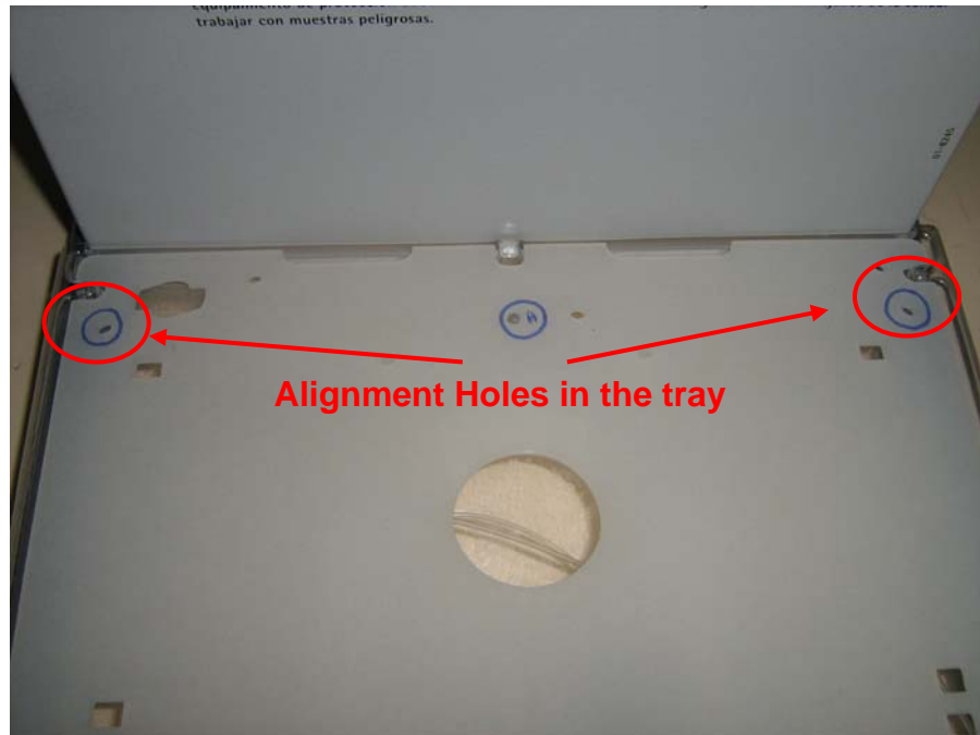
Figure 49. Holes in the Plate to Calibrate Point A
