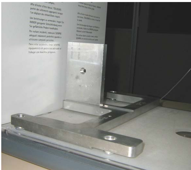
Figure 50. Alignment Tool in Position to Calibrate Point A
