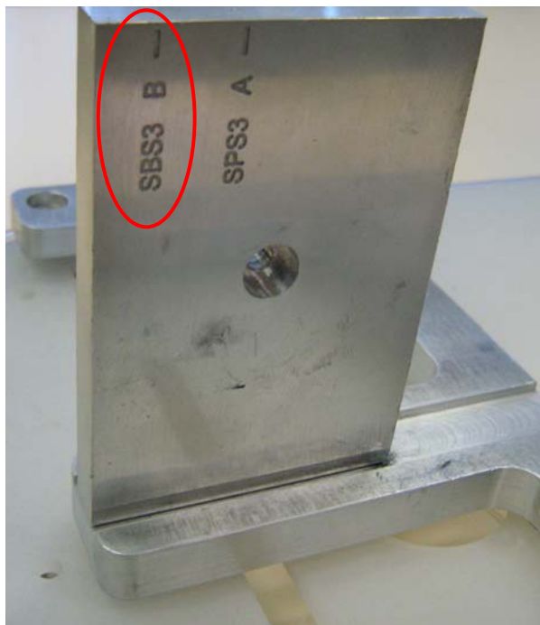
Figure 55. Calibration Point B in the Alignment Tool
