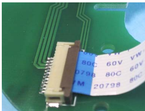
Figure 24. PCB cable connected
