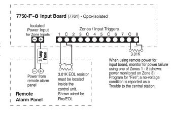
the zones as a power fail report. Install a 3.01K resistor on the designated zone terminals. Program the zone for F / Fire. When power to the input board is lost, zone will report a "Trouble". Flag this as a power failure at the central station / automation software.
