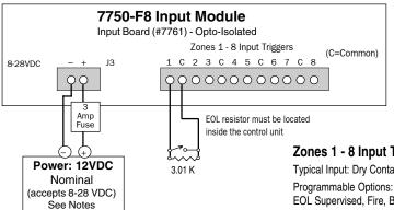
To monitor power on Input Board when powered by an alarm panel: For all Commercial Fire, UL burglar and Canadian UL burglar alarm installations, use one of the zones as a power fail report. Install a 3.01K resistor on the designated zone terminals. Program the zone for F / Fire. When power to the input board is lost, zone will report a "Trouble". Flag this as a power failure at the central station / automation software.
