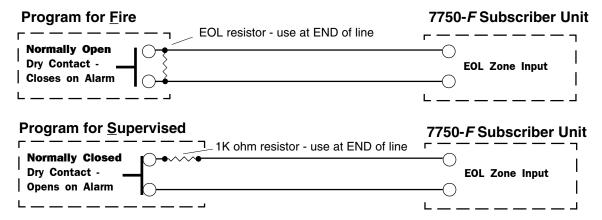
7750-F-4x4 NOTE: Maximum resistance of E.O.L. input, including wire and EOL resistor, is 1100 ohms. Thus, when using the 1K ohm resistor supplied, wire resistance must not exceed 100 ohms.
