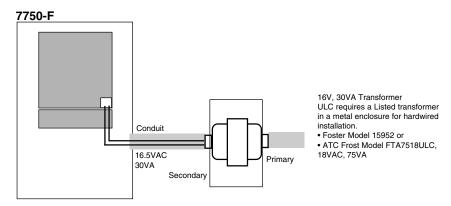
For cUL or ULC listed installations, the transformer must be permanently wired to its electrical outlet, or main power connection. It must be housed in a suitable metal enclosure, Listed for use in Canada, and that is provided with conduit connections. Suggested Transformers: Foster Transformer model 15952, or ATC Frost model FTA7518ULC. The transformer may be mounted inside the case of the 7750-F, if space allows.
