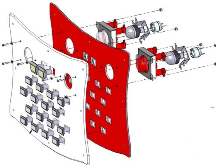
Remove these buttons to remove bulb socket bracket.
