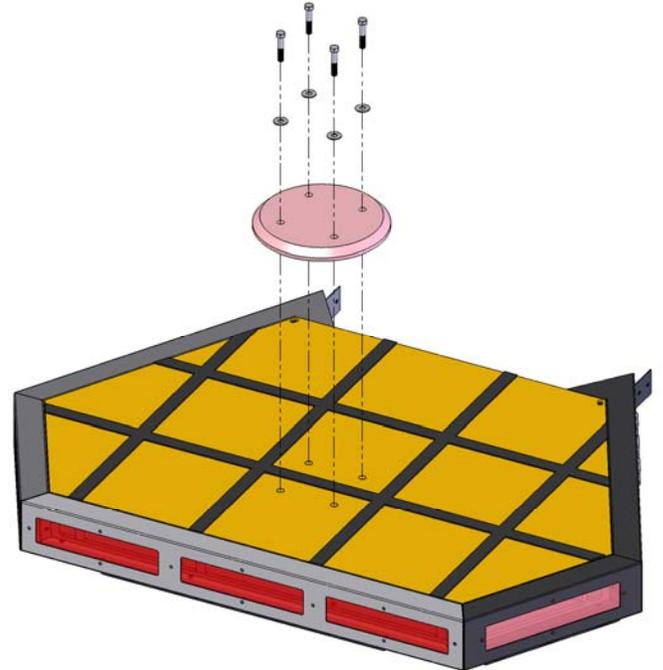
Remove the anti-slip tape from the platform to expose the fourteen screws that attach the floor to the stage. Now remove the floor. You can now access the fluorescent bulbs.
