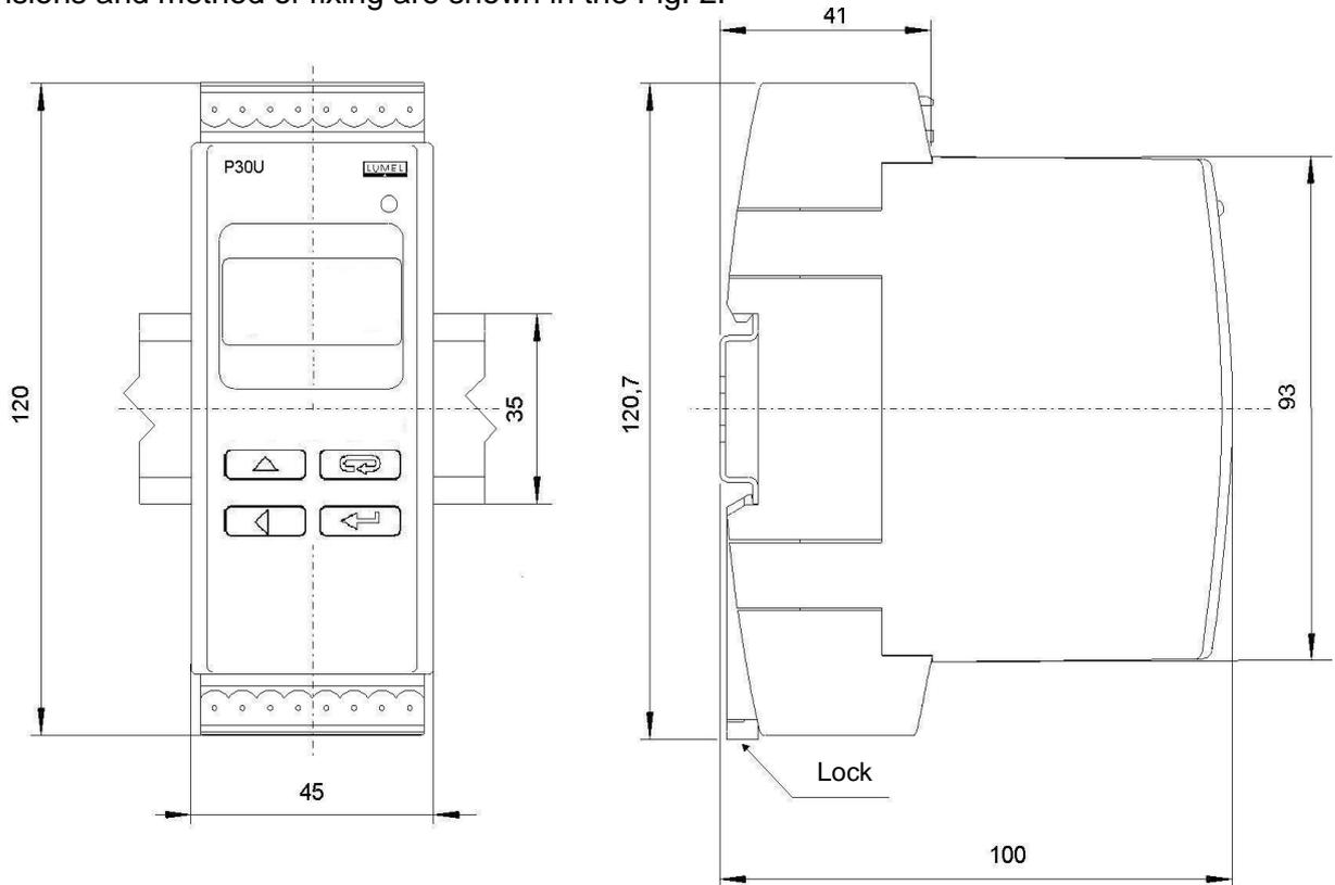
Fig. 2. Overall dimensions and method of fixing P30 transducers
