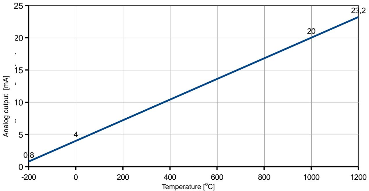
*Fig. 10. Work of the analog output when overflow options are switched off*
