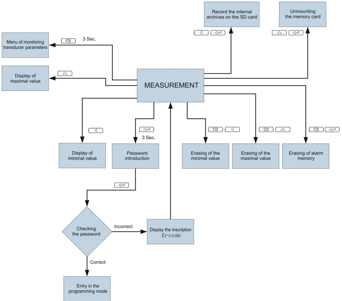
Fig. 5. Operation algorithm of the P30U transducer
