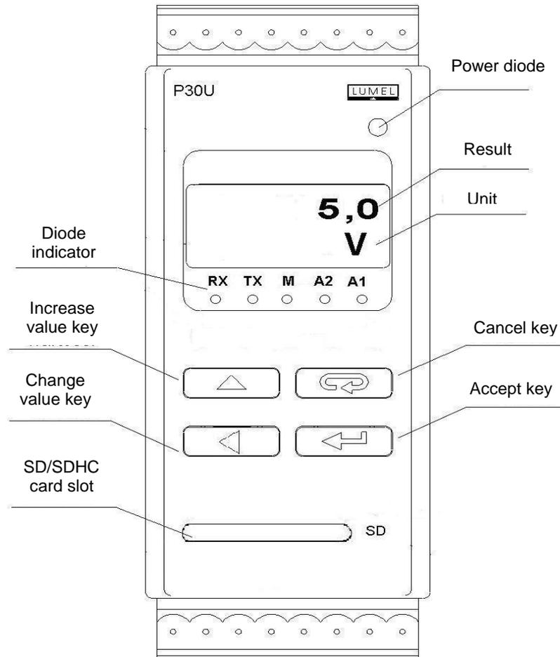
Fig. 4. Description of the transducer front panel
