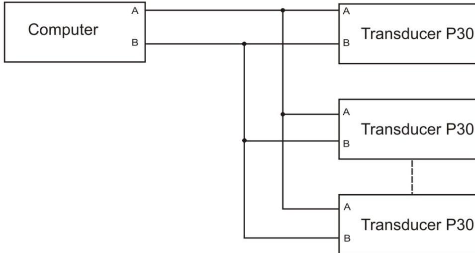
Fig.23. Method of connecting the RS-485 interface.
