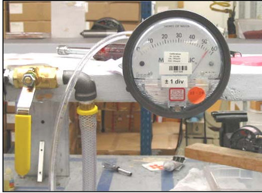
Figure 30. Magnehelic Gauge Connection to Hose Barb
