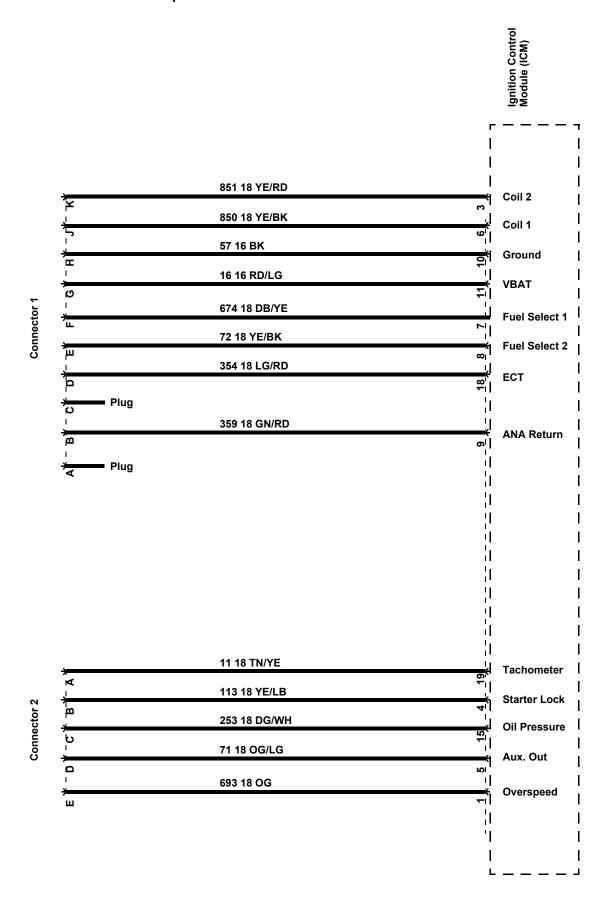
Engine Controls - Sensors & Data Link Connector (DLC) - ICM Jumper Patch Harness
