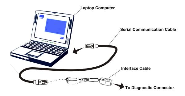
For connection to a PDA, use kit PN 2U1E-6K947-AA. Connect as shown below:
