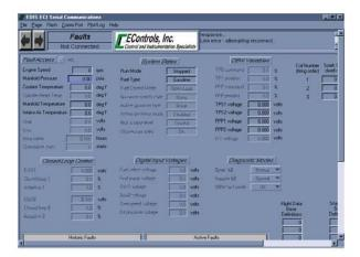
The Spark Kill diagnostic mode allows the technician to disable the ignition on individual cylinders. If the Spark Kill diagnostic mode is selected with the engine running below 1000 RPM, the minimum throttle command will lock into the position it was in when the test mode was entered. If the Spark System Test mode is selected with the engine running above 1000 RPM, the throttle will continue to operate mormally.
