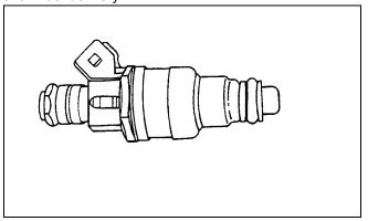
The fuel is injected under pressure in a conical spray pattern at the opening of the intake valve. Excess fuel
