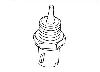
After engine start-up, the temperature should rise steadily to about 85°C (185°F). It then stabilizes when the thermostat opens. If the engine has not been run for several hours (overnight), the engine coolant temperature and intake air temperature displays should be close to each other. A fault in the engine coolant sensor circuit will set a DTC 221 or DTC 222.
