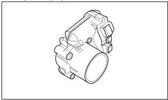
The Electronic Actuator also acts as an idle air control (IAC) valve. Changes in engine load are detected by the EPM by comparing manifold absolute pressure (MAP) with throttle position. When the EPM detects a change in engine load, it can adjust idle speed by changing the PWM signal to the actuator.
