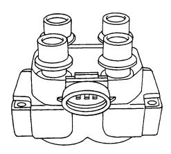
The primary coils in the coil pack are triggered by the "ignition coil feed#1" and ignition coil feed #2" signals from the EPM.
