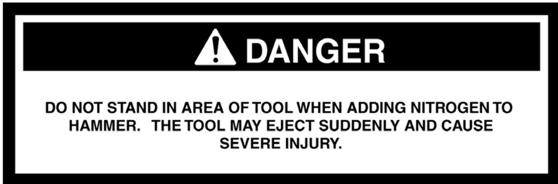
Make sure that the piston is positioned at the lower end of its stroke before charging. The piston and the cylinder may be damaged during gas charging by sudden movement (due to a pressure increase) if the piston is not at the bottom of its stroke in the cylinder.
