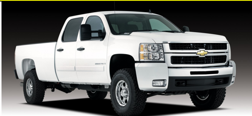
Shown: New Body 2007 Silverado 3500HD with 285/65R18 BFG T/A KO on 18"x 9" wheel with 5.0" of backspace.
