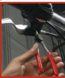
4. Remove the pivot pin, stock clutch lever, and the plastic clutch cable pin. Save these parts, they will be reused.
