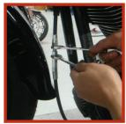
3. Using a snap ring pliers remove the retaining ring from the pivot pin located on the underside of the clutch pivot housing. Save the retaining ring, it will be reused.
