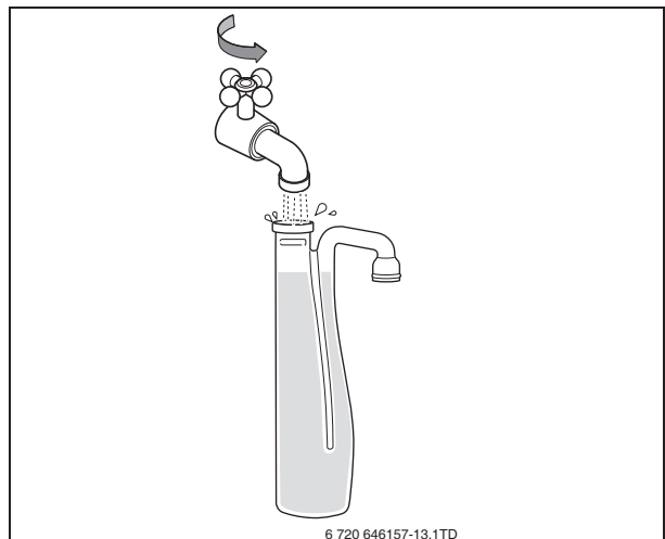
Fig. 13 Filling the condensate trap with water
