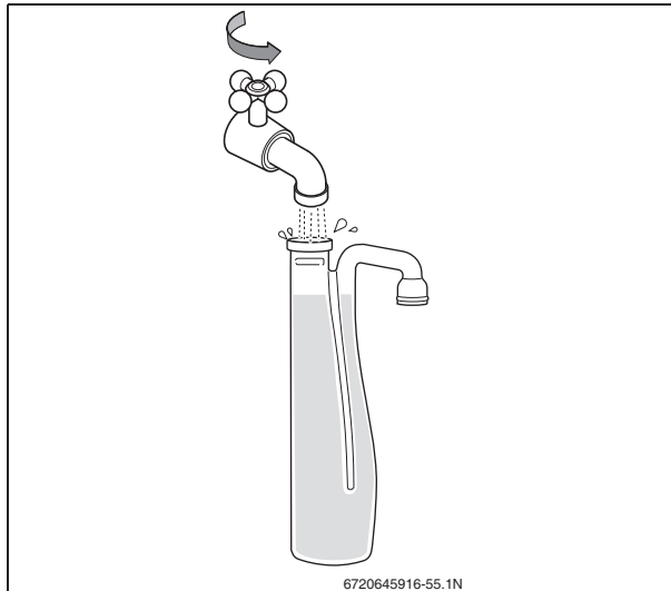
Fig. 55 Filling the condensate trap with water
