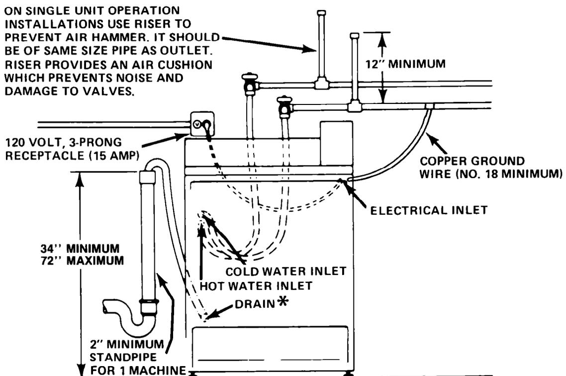
\*The drain hose assembly must fit in the standpipe so that there is an air gap around the drain hose inside the standpipe. A snug fit can cause a siphoning action.
