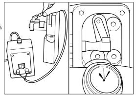
If any of three test results are outside specified value replace actuator by refering to *Actuator Replacement*.
