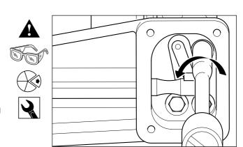
Carefully slide actuator rod from slot location with pivot block.
