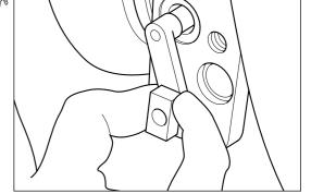
If pivot block rotates freely, remove pivot block and check linear travel of VG cross shaft pin is within permissible range shown in **Service Data Sheet**.
