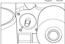
The sensor flange features a mechanical baulk (tab) to ensure correct sensor orientation.
