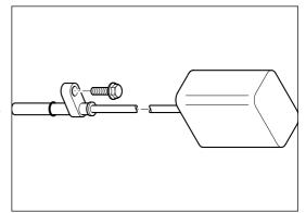
Where road spray, dirt and fluid ingress has caused fouling or corrosion of the speed sensor fastener apply a penetrating oil in accordance with the manufacturer's instructions.
