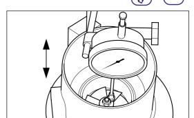
Check the radial movement at compressor impeller nose using a dial gauge.
