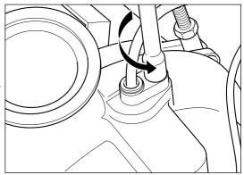
Extract the speed sensor ensuring that the o-ring seal is removed with the sensor. This is conveniently achieved by tilting the sensor as it exits its recessed bore.
