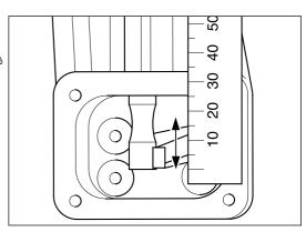
Apply system voltage to actuator motor through on/off switch. Switch voltage to retract and extend actuator rod. Check actuation cycle can be completed in 5 seconds.
