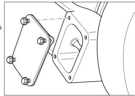
Using a calibrated torque wrench, torque tighten the 4 cap head screws to the value shown in the Service Data Sheet
