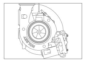
With intake system disconnected from compressor housing, it may be possible to check for excess bearing axial and radial clearances.
