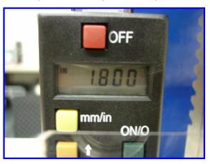
NOW YOU CAN INSPECT MULTIPLE SPRINGS USING THE 1" BLOCK FOR INSTALLED HEIGHT, THE .500 BLOCK FOR ½ LIFT HEIGHT AND NO BLOCK FOR FULL LIFT HEIGHT. YOU MUST BE CAREFUL NOT TO OVER PULL THE DEAD STOP AS IT IS NOT PINNED BUT A FRICTION STOP. THIS WILL TAKE SOME TIME TO GET USE TO. IF THE DEAD STOP BECOMES SLOPPY IN THE UNLOCKED MODE. THE SET SCREWS ON THE FRONT AND SIDE CAN BE READJUSTED TO A PERCEPTIBLE DRAG AND ELIMINATE THE SLOP.
