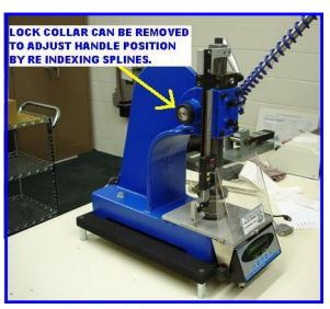
BOTH THE LINEAR AND LOAD DRO CAN BE SWITCHED INTO METRIC UNITS OF MEASURE WITHOUT THE NEED TO RE ZERO OR RE CALIBRATE. ANY COMBINATION IS ALSO POSSIBLE. KG FORCE WITH INCH HEIGHT OR LBS FORCE WITH MM HEIGHT.
