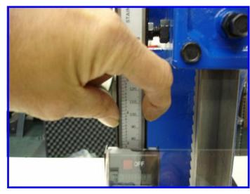
IF THIS DOES NOT CORRECT THE PROBLEM THEN CHECK THE ALIGNMENT OF THE SCALE. THE BLACK REAR BRACKET MUST MOVE PARALLEL TO THE ARBOR SHAFT. THIS CAN BE VERIFIED VISUALLY BY MOVING THE HANDLE UP AND DOWN WHILE OBSERVING THE REAR BRACKET IN RELATION TO ONE OF THE FREE PLAY BOLTS IN THE LEFT HAND SIDE OF THE ARBOR HEAD. IF IT DOES NOT MOVE PARALLEL, THEN LOOSEN AND ADJUST THE UPPER BRACKET SCREWS. (see picture below)
