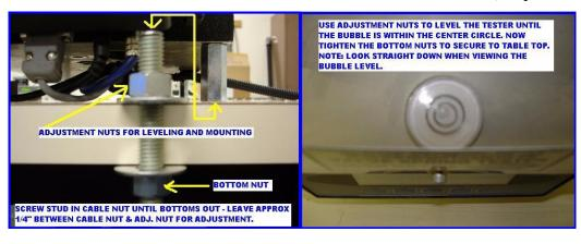
LOOKING STRAIGHT DOWN - THROUGH THE LEXAN SHIELD -ADJUST THE ADJUSTMENT NUTS UNTIL THE BUBBLE IN WITHIN IN INNER CIRCLE.
