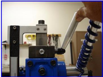
THE DEAD STOP IS EQUIPPED WITH TEFLON BUSHINGS AND CAN BE PRE LOADED WITHOUT DAMAGING THE SURFACES OF THE ARBOR SHAFT. OW YOU CAN PULL THE ANVIL DOWN TO THE LOWEST DESIRED HEIGHT AND LOCK IT IN PLACE.
