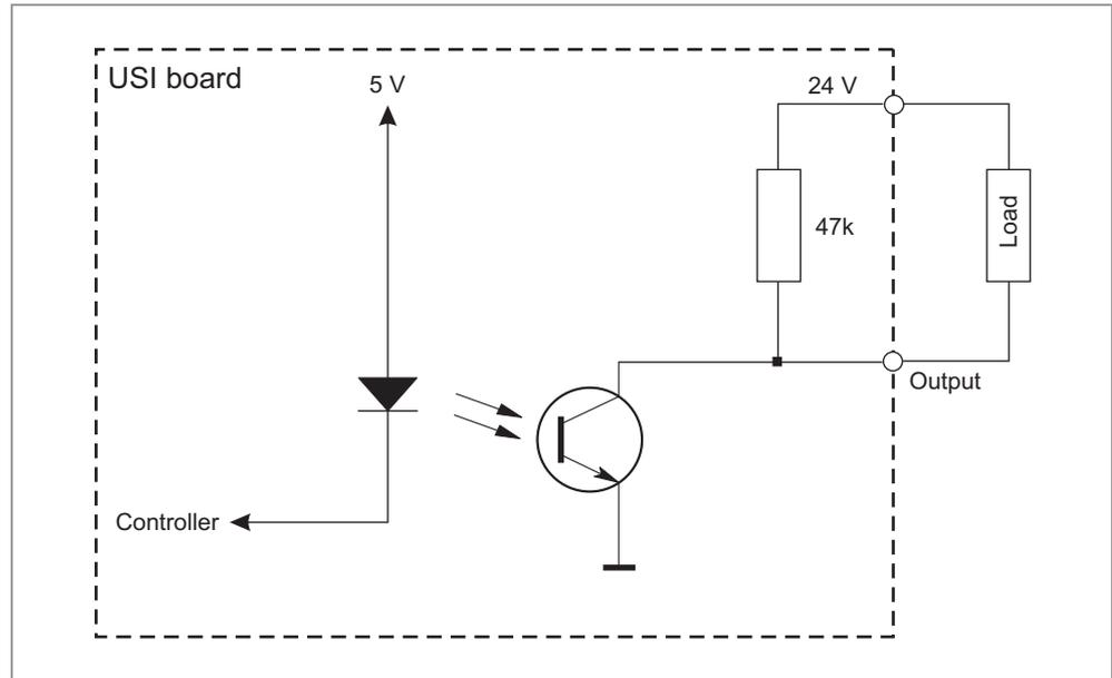
[9] Main circuit (NPN) for signal outputs at the USI interface.
