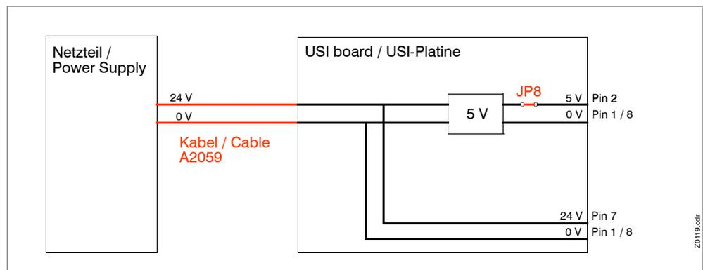
[10] USI in the state of delivery: The voltage cable is connected, JP 8 is closed.
