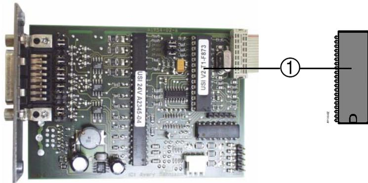
[11] The controller (1) contains the USI firmware.
