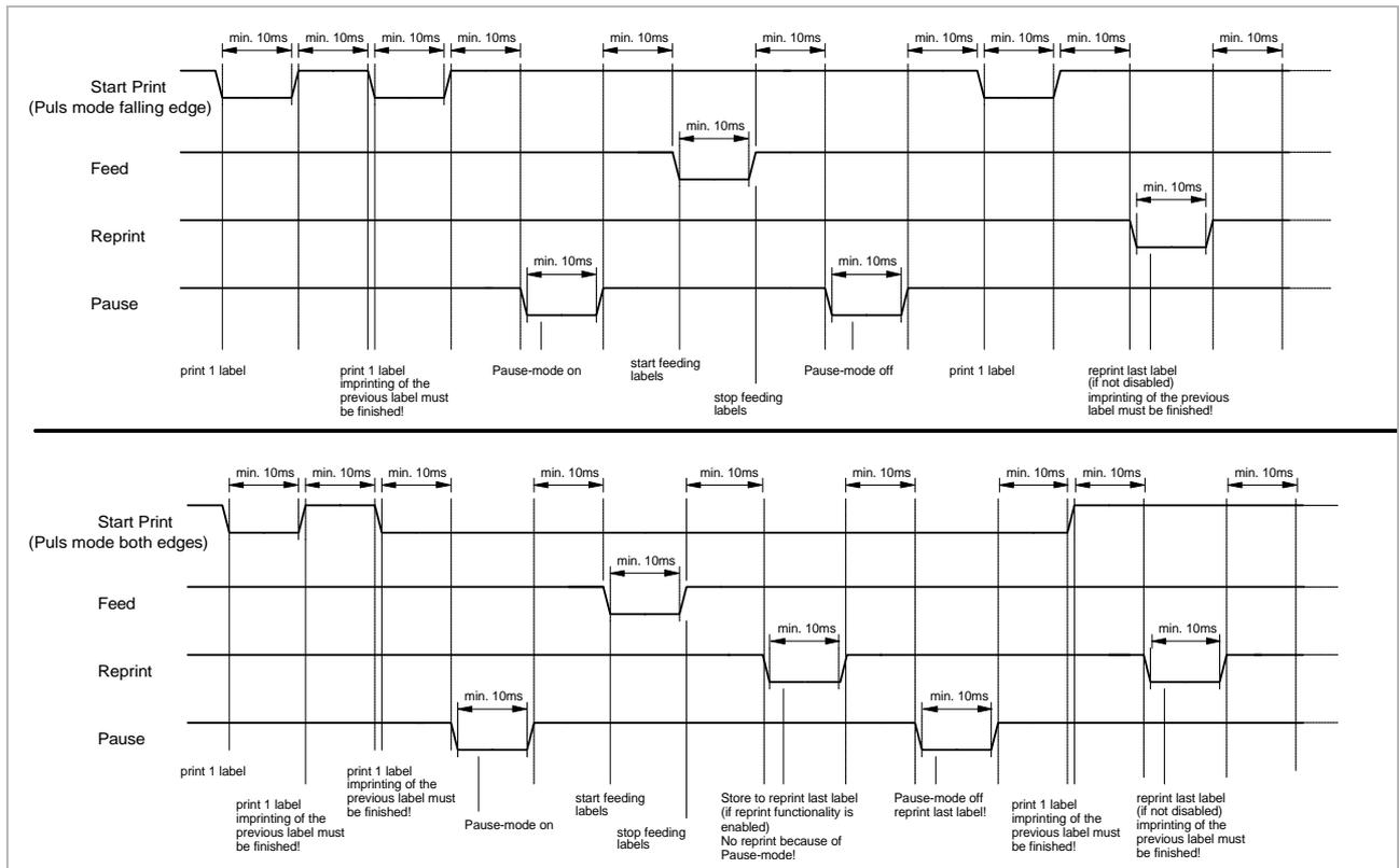
[7] Examples of timing waveform for the USI inputs.
