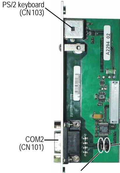
**L** CAUTION! The maximum output current of the PS/2 interface is 500mA at 25°C!
