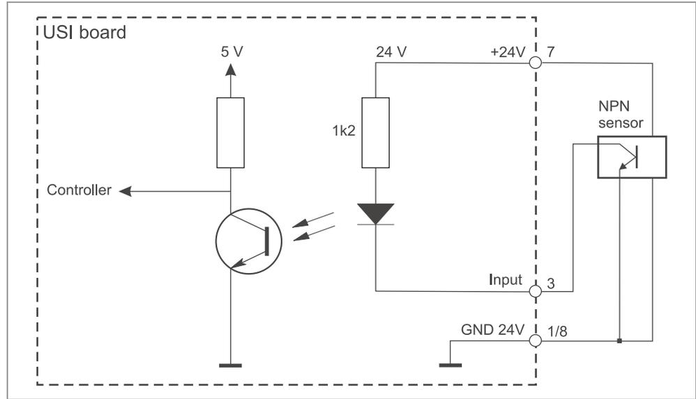
[6] Main circuit for signal inputs (NPN) at the USI interface (here: connecting a start sensor).
