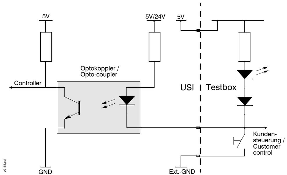
Fig. 16: Simplified diagram of a USI input.
