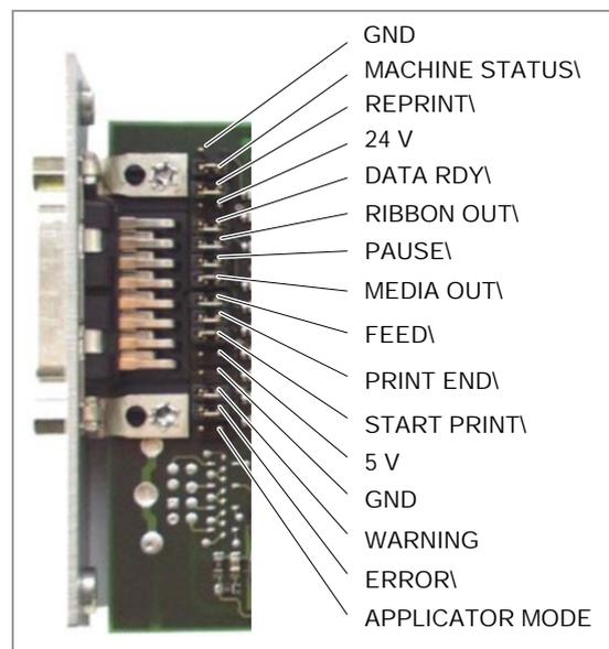
[4] Pin assignment jumper block
