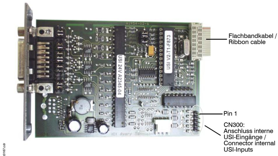
Fig. 15: Pin 1 is the first pin in direction of the ribbon cable; the writing CN300 Pin 1 can be found beside the pins on the USI board.
