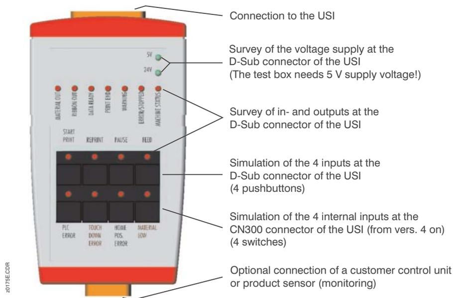
Fig. 13: Operating parts and connections of the USI testbox.
