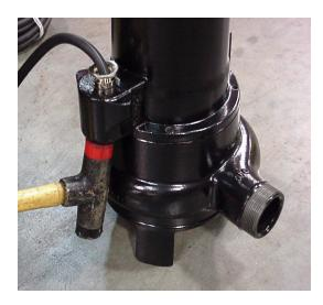
Sometimes the housing will be difficult to remove. Twist the housing ¼ turn (90 degrees), exposing the bottom of the cable entry horn. Using a soft faced hammer, gently tap the cable entry horn to free the stator housing.
