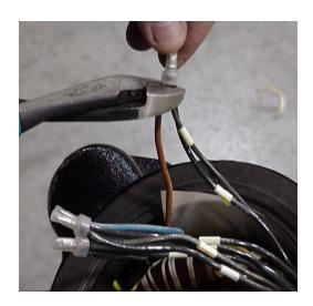
To perform the reconnection, locate the wire bundle with wires 1, 7, and the power lead. Cut wire connector from the bundle, freeing individual wires. Strip wire sheathing back <sup>1</sup>/<sub>4</sub>" in preparation for reconnection.
