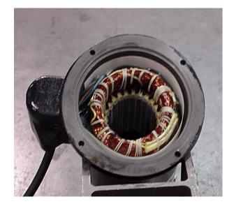
6. With motor disassembled, turn stator housing upside down, and support it so it is free standing. Stator windings and cable leads must be visible and easy to reach. Your unit should now look like this. **Gently** remove all wires from around the stator windings. Take care not to damage the winding insulation. **Do not use sharp tools!!**
