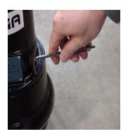
2. With pump in stable, upright position, remove the 5mm cap screws as indicated.
