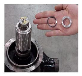
5. With stator housing removed, determine if a wavy washer is present by checking the top of the bearing, the top of the stator housing, and the stator windings. Place it aside until reassembly.
