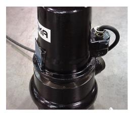
Carefully lift stator housing 3 inches with hoist, if available, and check under stator housing for internal seal probe.
