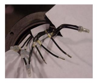
Now you should have three new bundles 2 and power 3 and power 1 and power along with 3 separate wires (#7,#8,#9), and one bundle of 3 wires (#4,#5,#6). 13. Now, you will need to separate the wire bundle with numbers 4, 5, 6, and pair each wire with the loose wires numbers 7, 8, and 9 as indicated. Using the last three wire connectors:
