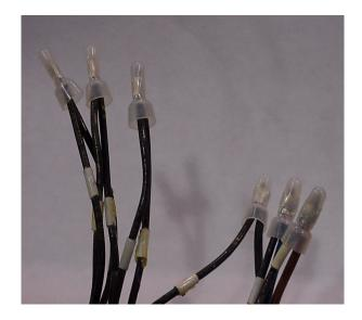
14. At this point, you should have 6 separate wire bundles, each with 2 wires. Wires should be paired as follows: 4 to 7, 5 to 8, 6 to 9, #1 to power, #2 to power and #3 to power.
