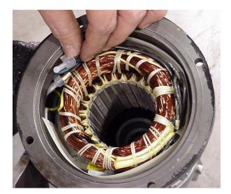
15. Starting with bundles 4-7, 5-8, 6-9, gently tuck these 3 wire bundles behind the windings on one side of stator. Then tuck the remaining 3 bundles behind the windings on the other side. Take care that all wires are tucked between stator winding and housing. Also check that white phase paper is in proper position, and not extending below the stator housing.
